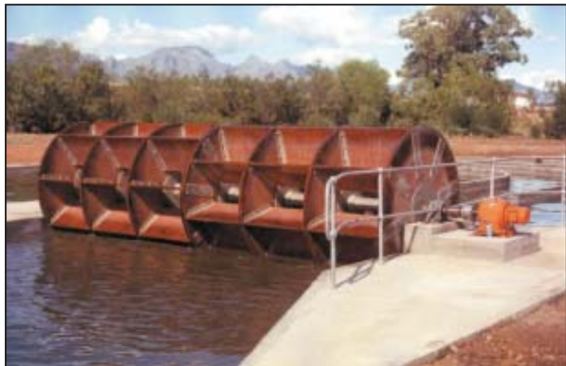
An impressive paddle wheel keeps the water flowing steadily round the 2 500 m 2 high rate algal pond at the Wellington tannery where Spirulina biomass is produced commercially today.
