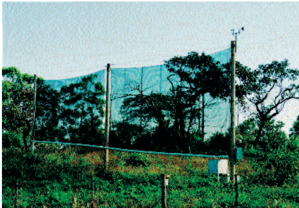
The giant fog screens at Tshanowa Junior Primary School in Limpopo province are providing pupils and members of the community an average of between 150ℓ and 250ℓ of water per day.
