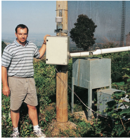
Hannes Rautenbach, of the University of Pretoria's Department of Geography, Geoinformatics and Meteorology, beside one of the 36 m 2 screens. Water drips from the net into a gutter, and runs through a sand filter before being channelled into the storage tank. The automatic weather station (the white box) records rainfall, wind speed and wind direction.
