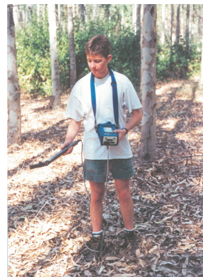
Dave Drew ,Author , measuring the leaf area of Eucalyptus stands with an instrument that measures light interception beneath the canopy
