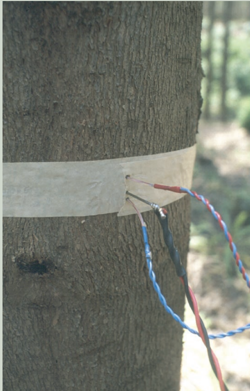
The heat pulse technique was used to measure the flow of sap in the sapwood of the tree
