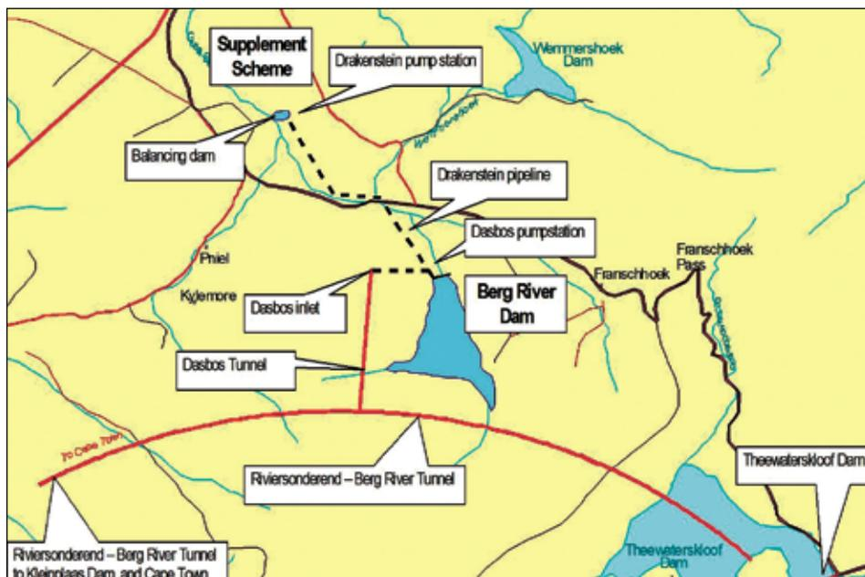
*The Berg Water Project comprises the Berg River Dam (which is about 6 km west of Franschhoek) and the Supplement Scheme situated about 12 km downstream. The latter comprises a 1,6 m-high diversion weir that diverts a portion of the winter high flows into a 3 ha off-channel balancing dam from where the water is pumped via a 12 km pipeline back into the Berg River Dam.*
