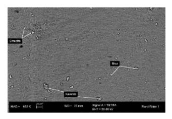
Figure 1 An electron backscatter image of the sample surface at relatively low magnification
