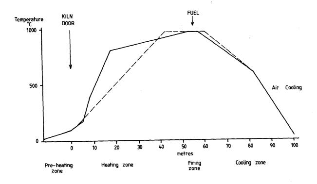
Figure 2 Kiln temperature profile
