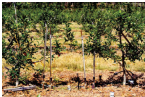
Right: Field tests: Tensiometers and neutron probes.
