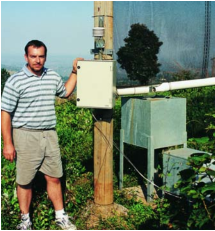
Hannes Rautenbach, of the University of Pretoria's Department of Geography Geoinformatics and Meteorology, beside one of the 36m screens. Water drips from the net into a gutter and runs through a sand filter before being channelled into the storage tank. The automatic weather station (the white box) records rainfall, wind speed and wind direction.
