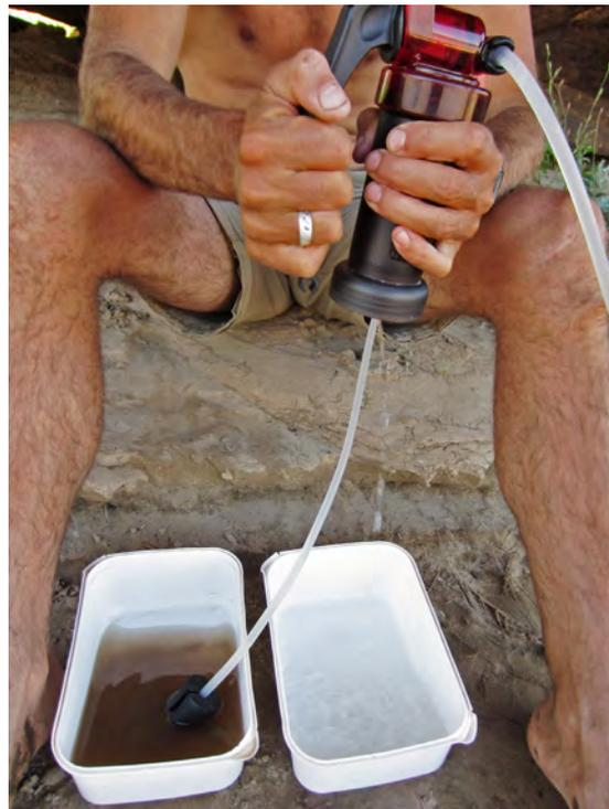
An example of dirty unfiltered water (left) and clean filtered drinking water (right).
