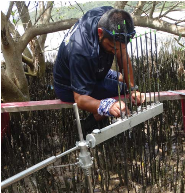
Oceanographic technician Imtiyaz Malick (SAEON) checks an RSET installation at Nahoon Estuary.
