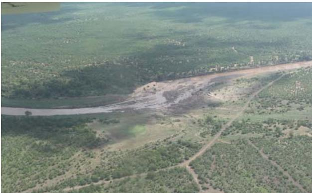
*The Kanniedood Dam before, during and after demolition in 2018/19. The dam was removed completely after the wall was breached by flood in 2013, causing the river to open a new channel bypassing the dam wall on the southern bank of the Shingwedzi River.*
