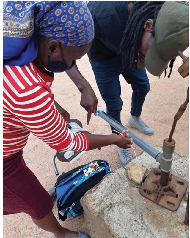
*Citizen scientists using a dip meter to measure water levels of boreholes in Limpopo's Hout catchment area.*
