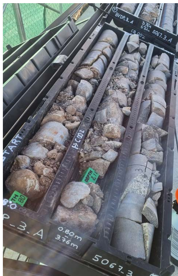
Core trays containing the first core from the borehole. The WRC-funded project managed to drill to 950 m before its time at the site came to an end; however, drilling continued as part of the larger Bushveld Complex Drilling Project.
