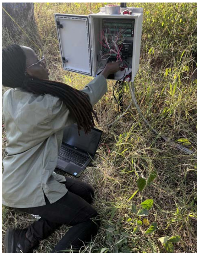
Project team member Mashudu Makhado installing the heat ratio sap flow method for measuring transpiration at the Phalabowa study site.
