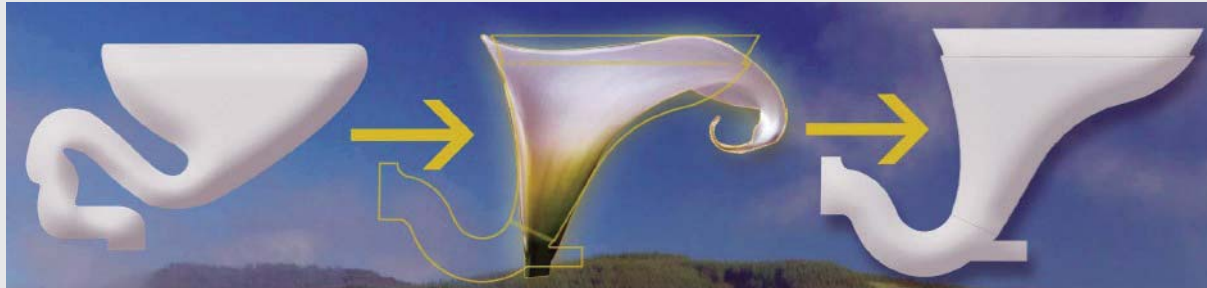
Figure 6: Arumloo low (micro) flush toilet
