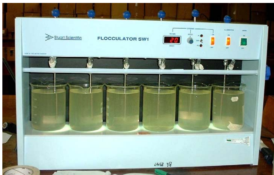
Fig.4 .4 Jar test apparatus
