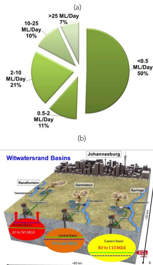
Figure 2: Distribution of the (a) WWTW capacity within the South African wastewater sector and (b) schematic for the mine-impacted water treatment works within the Witwatersrand basin
