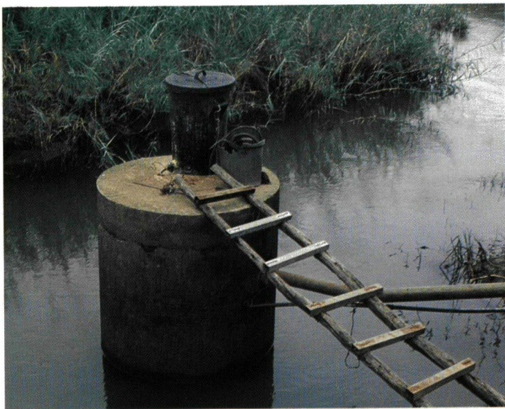
A 100 litre volume water sample being taken at a protected borehole.
