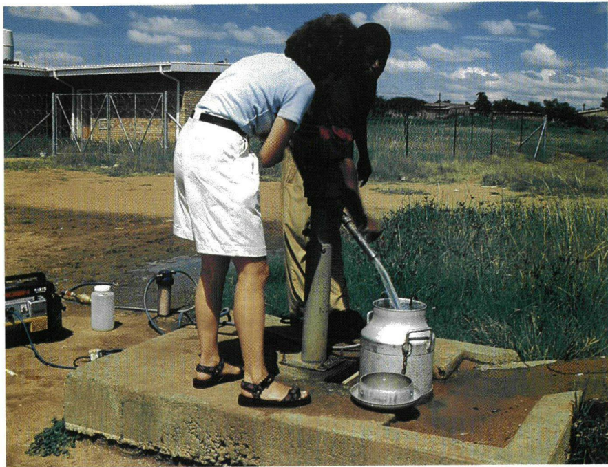
A 100 litre volume water sample being taken at a protected borehole.
