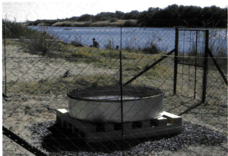
Land-based A-pan evaporation data was used in a 1988 study to estimate the evaporation losses from the Orange River.
