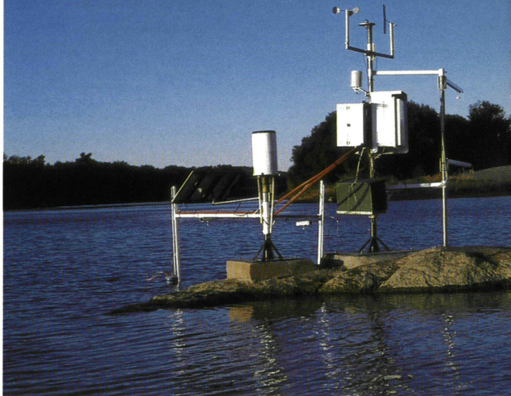
The Bowen ratio apparatus sited on a small outcrop in the middle of the Orange River, ten kilometres upstream from Upington in the Northern Cape.
