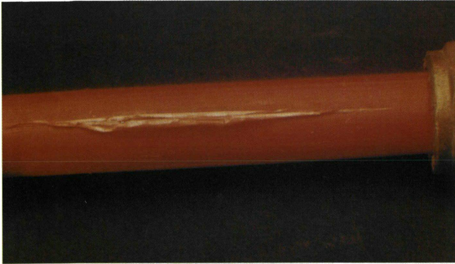
A very bad extrusion resulting in a combination of ductile / brittle failure. An angled crack resulted ultimately in a ductile "ballooning."
