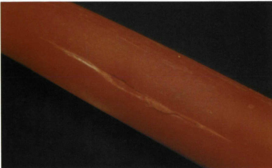
Brittle crack failure initiated by an indentation from a sharp rock.
