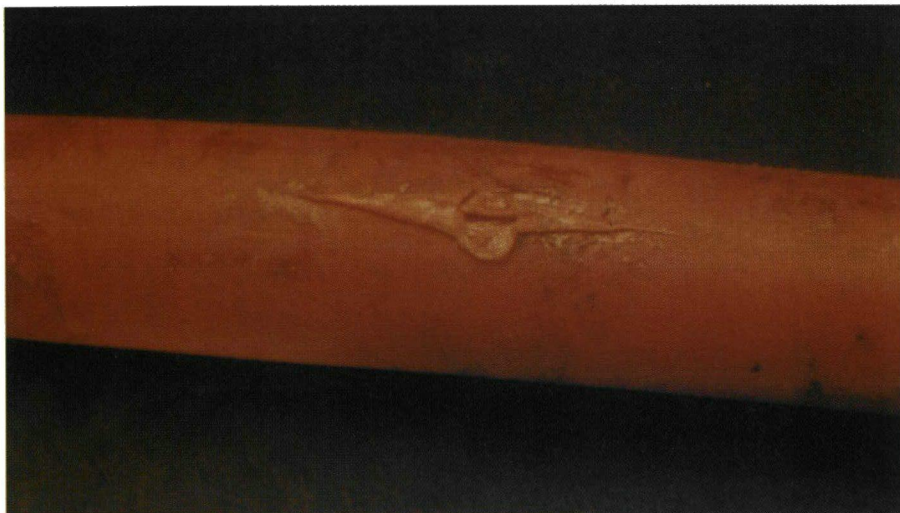
This pipe showed evidence of two brittle cracks inside and an eventual ductile failure on the outside.
