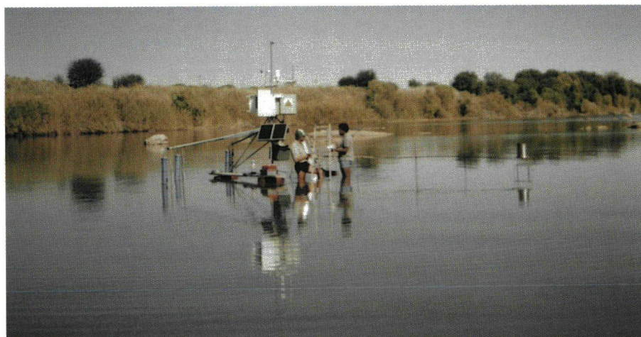
Bowen Ratio equipment used to measure evaporation from the Orange River surface
