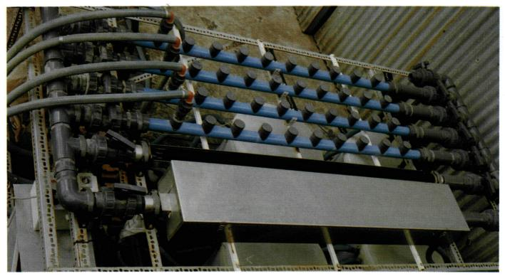
A view of the biofouling rig from above, showing the stainless steel box containing the UV irradiated channel and the open untreated channel (black area) next to the stainless steel box.
