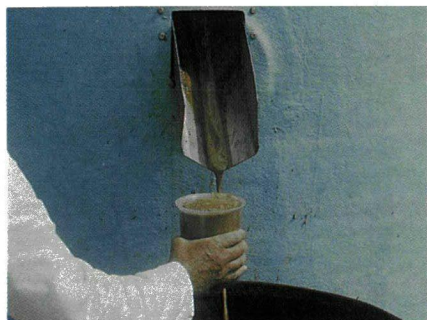
Wastes consisting principally of lipids (eg oleic acid) will not generate a pelletised sludge. Such wastes might generate a sludge bed, but of a gelatinous nature.
