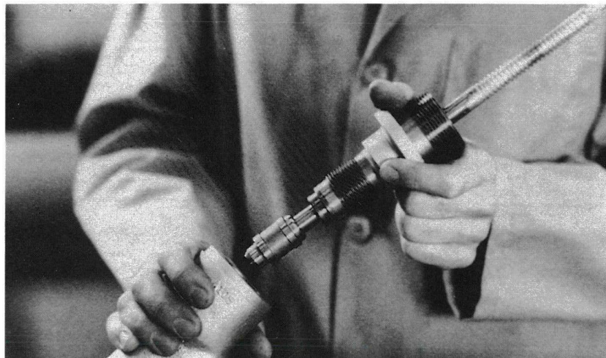
Removing the valve bonnet-stem-disc assembly of an Edward Univalve for maintenance. The valve body remains on-line.
