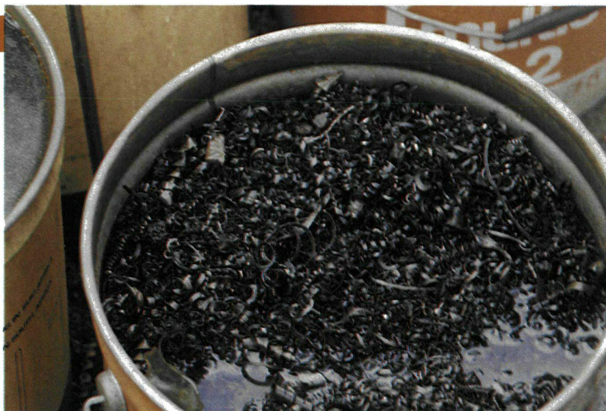
The iron filings used in the Catphate unit to remove phosphate from effluent.
