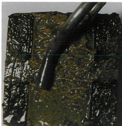
A mild steel sample showing microbially influenced corrosion (MIC) attack.
