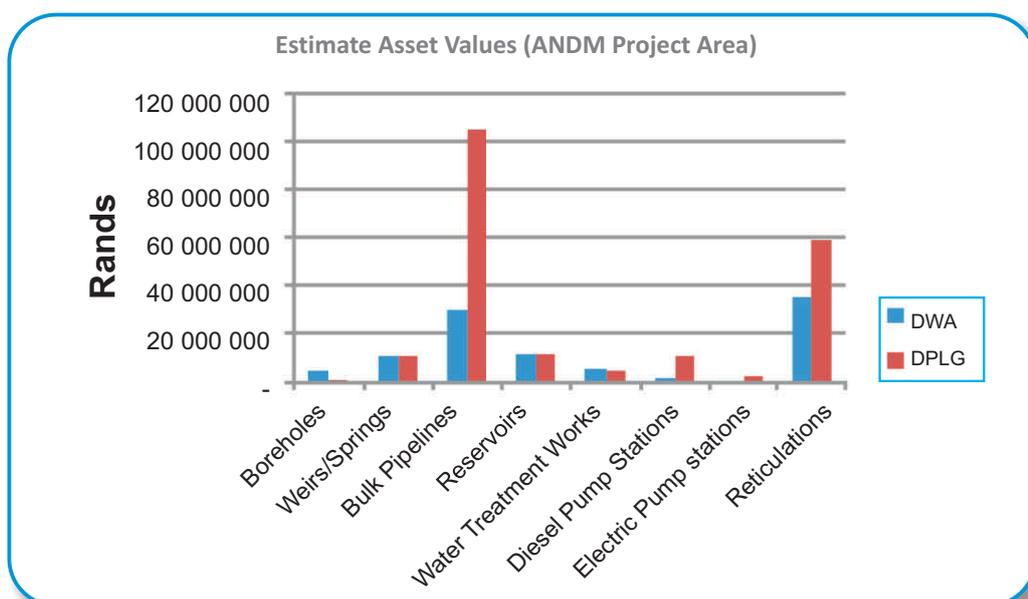
The chart shows that bulk pipelines, together with rising mains, constitute the single biggest asset cost component.
