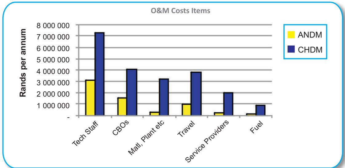
Materials and plant costs were much higher in CHDM because the project area has a far higher number of mech/elec installations with rotating equipment. These are far more prone to failure than static infrastructure such as pipelines and reservoirs.
