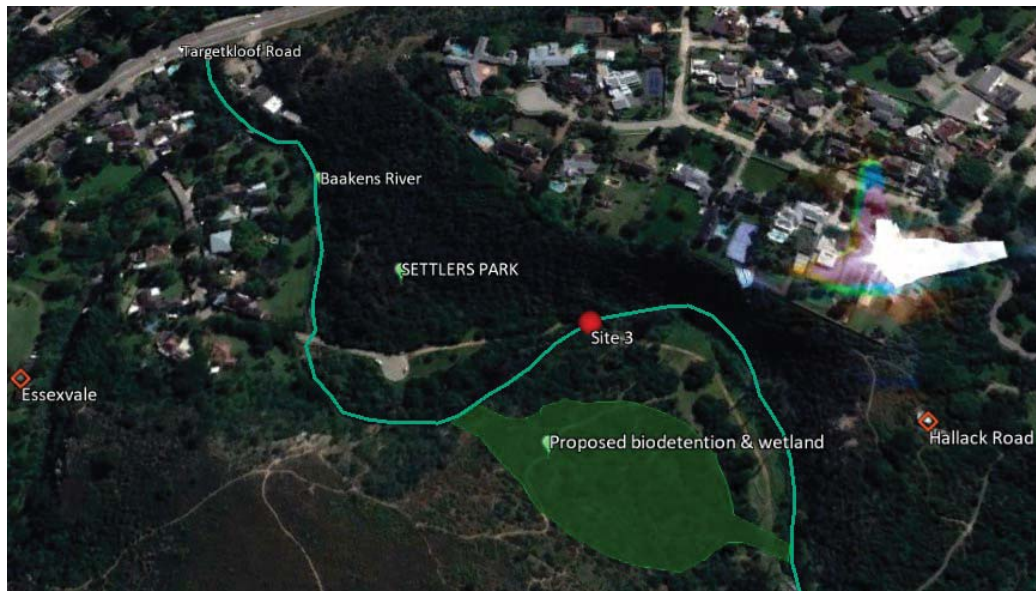
Figure 6.3 An optional location for one of the proposed bioretention ponds with a wetland component, downstream of an area demarcated as a flood hazard zone of the catchment. Within the Settlers Reserve. Note: The total surface area illustrated here is 14,000 m 2
