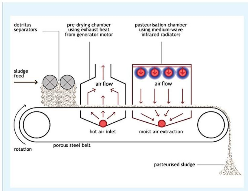
**Figure 2.7: Schematic representation of the LaDePa machine designed to process faecal sludge into pasteurised sludge. Adapted from Kengne et al. (2014).**
