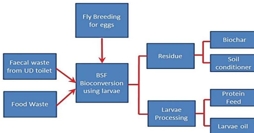
**Figure 2.6: Black Soldier Fly Larvae (BSFL) technology processing faecal waste from urine diversion (UD) toilets and food waste to produce marketable products (Mutsakatira et al., 2018).**
