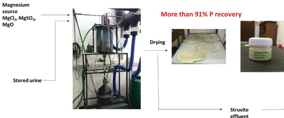
**Figure 2.3: The struvite production process. The reaction takes place in the automated reactor shown on the left.**
