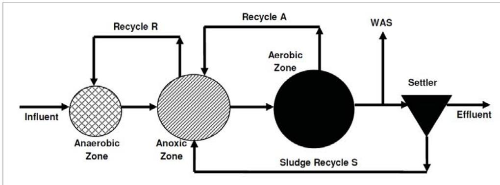
Figure 2-3: Diagrammatic layout of the UCT process (adapted from Ekama et al., 1984)
