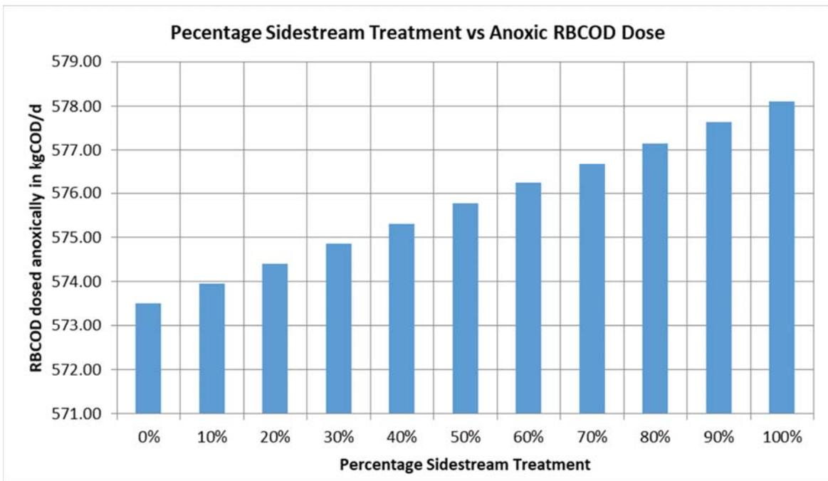
Figure 76: Impact of side-stream treatment on required RBO for use in anoxic zone, for NO<sub>3</sub> removal at 'D' WWTP
