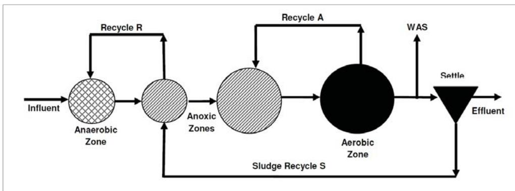
Figure 2-4: Diagrammatic layout of Modified UCT process (adapted from Ekama et al., 1984)
