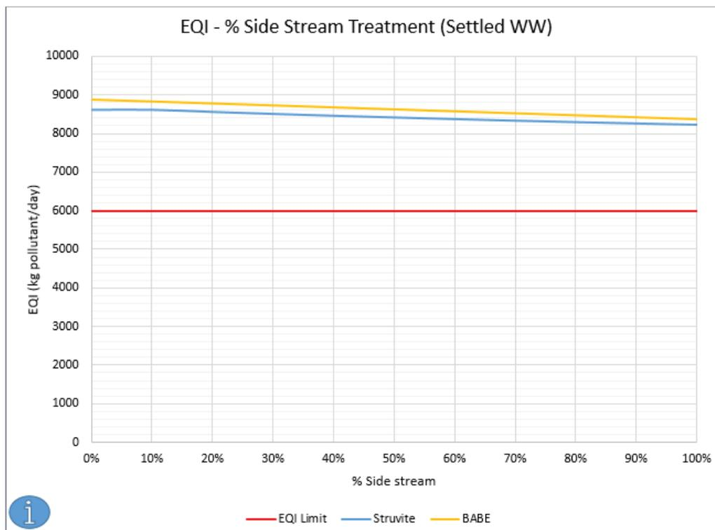
Figure 5-7: EQI variation with the percentage of dewatering liquor treated for plant A
