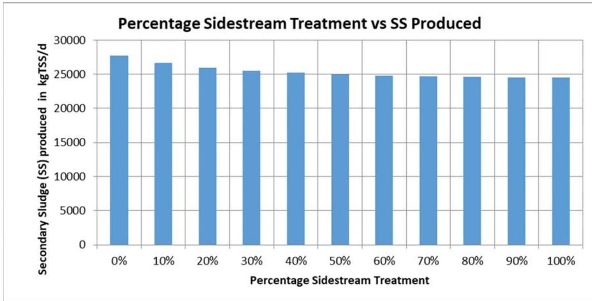
Figure 59: Impact of side-stream treatment on secondary sludge production at 'C' WWTP
