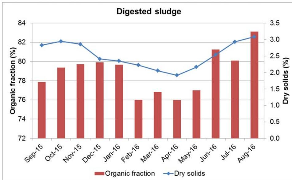
Figure 67: Monthly average organic fraction and dry solids content in the digested sludge at 'C' WWTP
