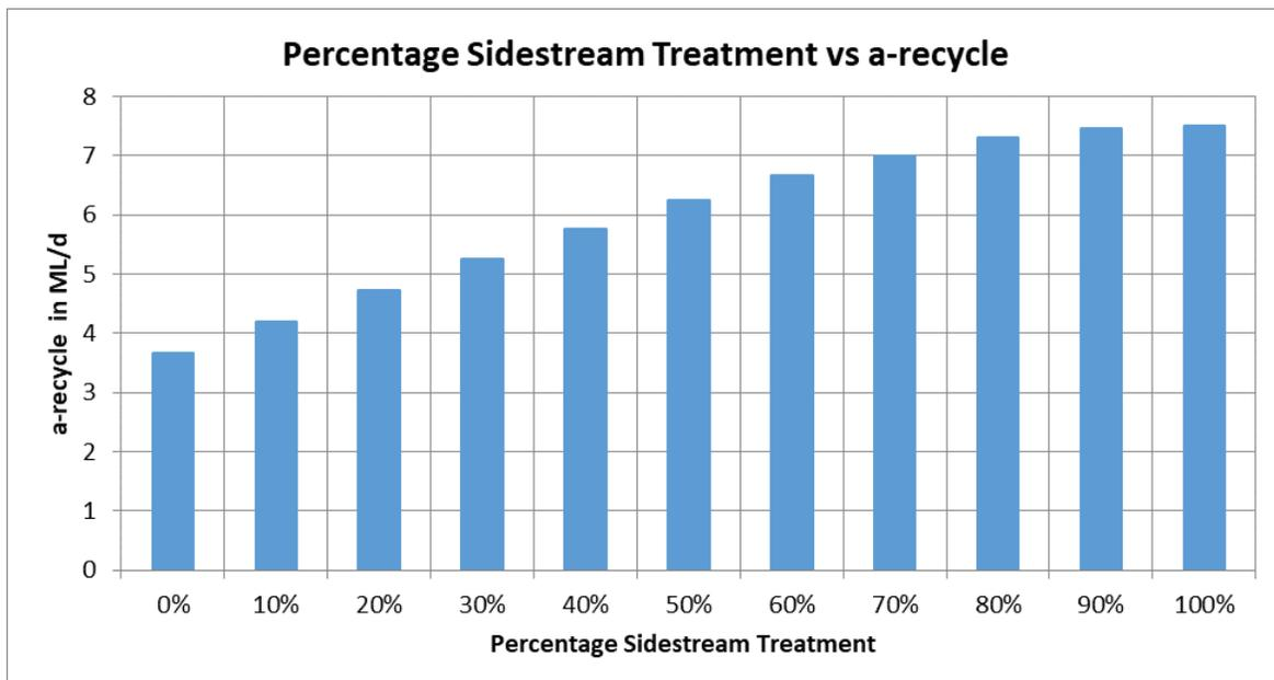
Figure 19: Impact of side-stream treatment on Module 2 a-recycle at 'Z' WWTP
