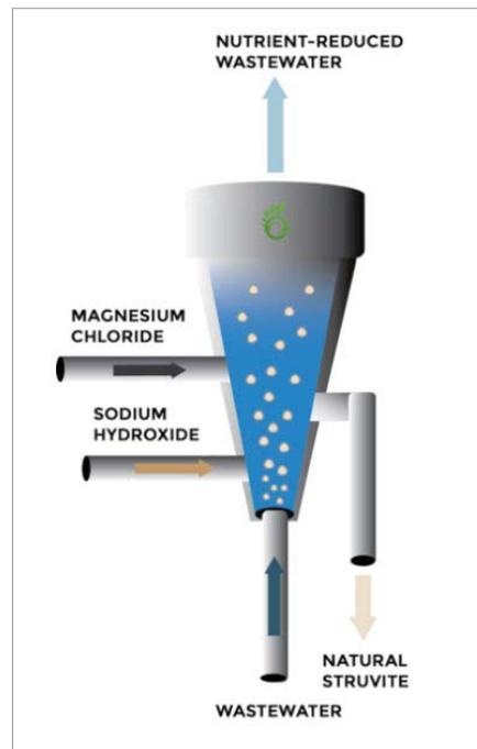
Figure 2-9: Multiform Harvest™ struvite reactor (Multiform Harvest, 2015)
