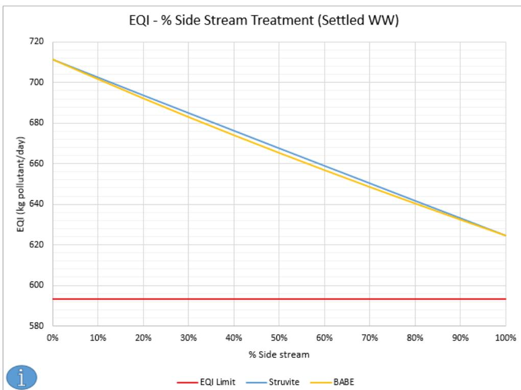
Figure 5-9: EQI variation with the percentage of dewatering liquor treated for plant C
