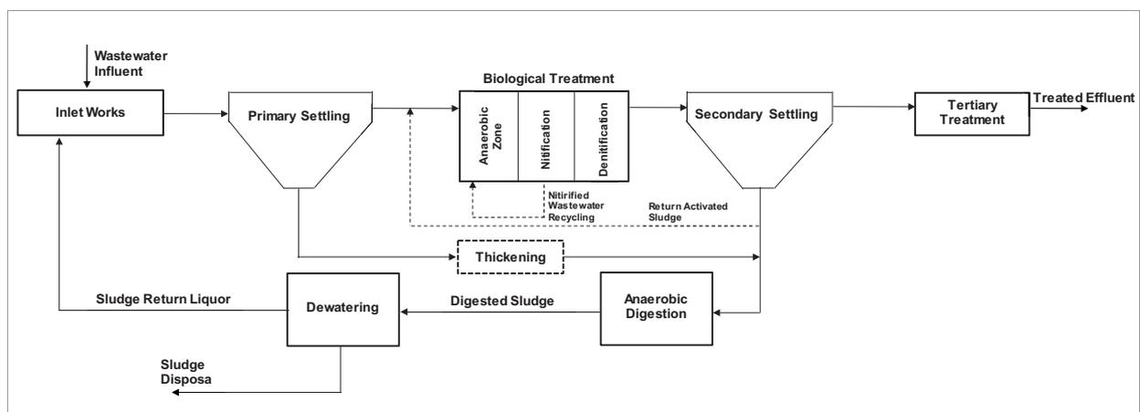
Figure 2-1: Typical wastewater treatment process
