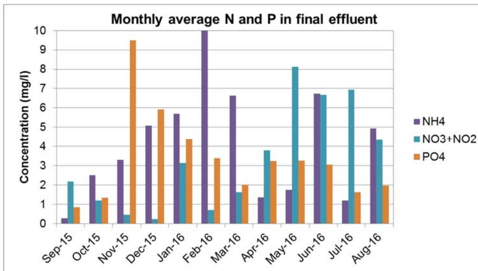
Figure 76: Monthly average ammonia, nitrate+nitrite and orthophosphate in the final effluent at 'D' WWTP<sup>2</sup>
