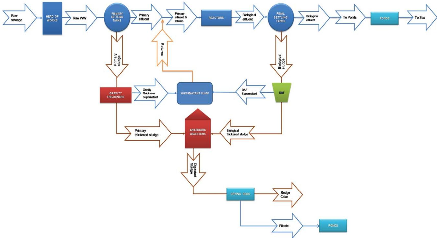
Figure 59: General process flow diagram of 'C' WWTP
