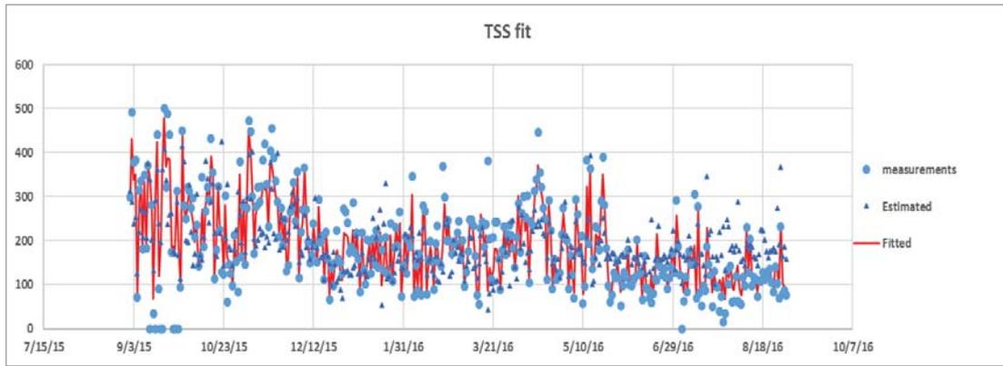
Figure 5-3: Comparison between measured, interpolated and fitted TSS values
