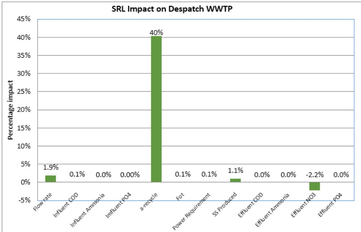
Figure 77: SRL impact on ‘D’ WWTP at 0% side-stream-treatment
