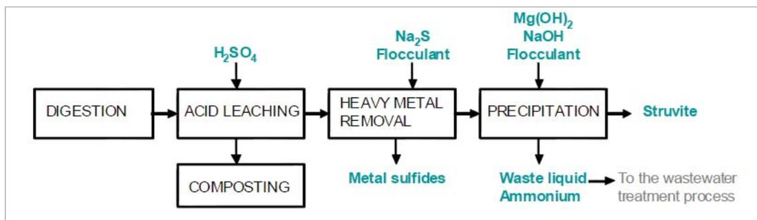
Figure 2-12: Flowchart for the Seaborne process at Gifhorn (Adapted from Nieminen, 2010)
