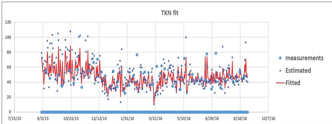
Figure 5-4: Comparison between measured, interpolated and fitted TKN values
