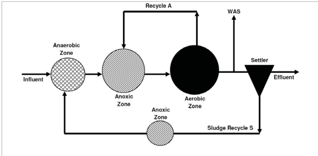
Figure 2-5: Diagrammatic layout of the JHB process (adapted from Ekama et al., 1984)
