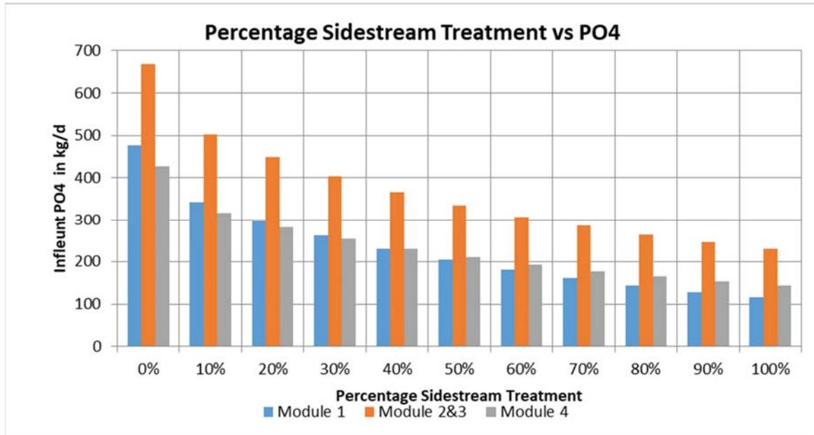
Figure 5: Impact of side-stream treatment on influent phosphate at 'W' WWTP
