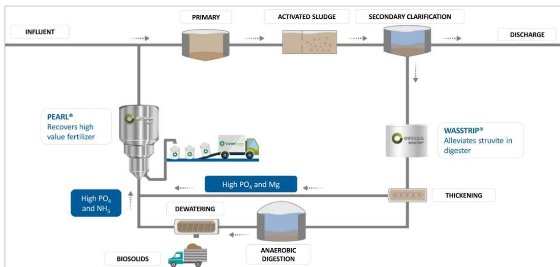
Figure 2-8: Synergistic use of the Ostara + WASSTRIP processes (Clark, 2017)
