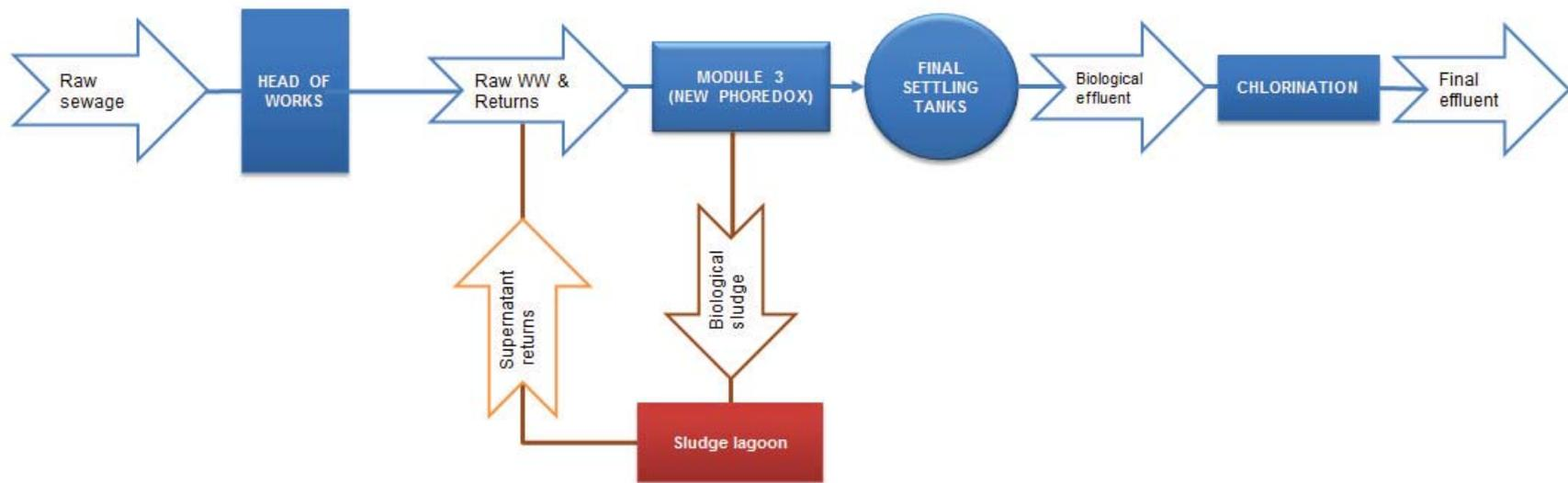
Figure 71: General process flow diagram of 'D' WWTP
