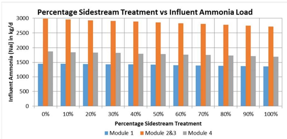
Figure 4: Impact of side-stream treatment on the influent ammonia at 'W' WWTP
