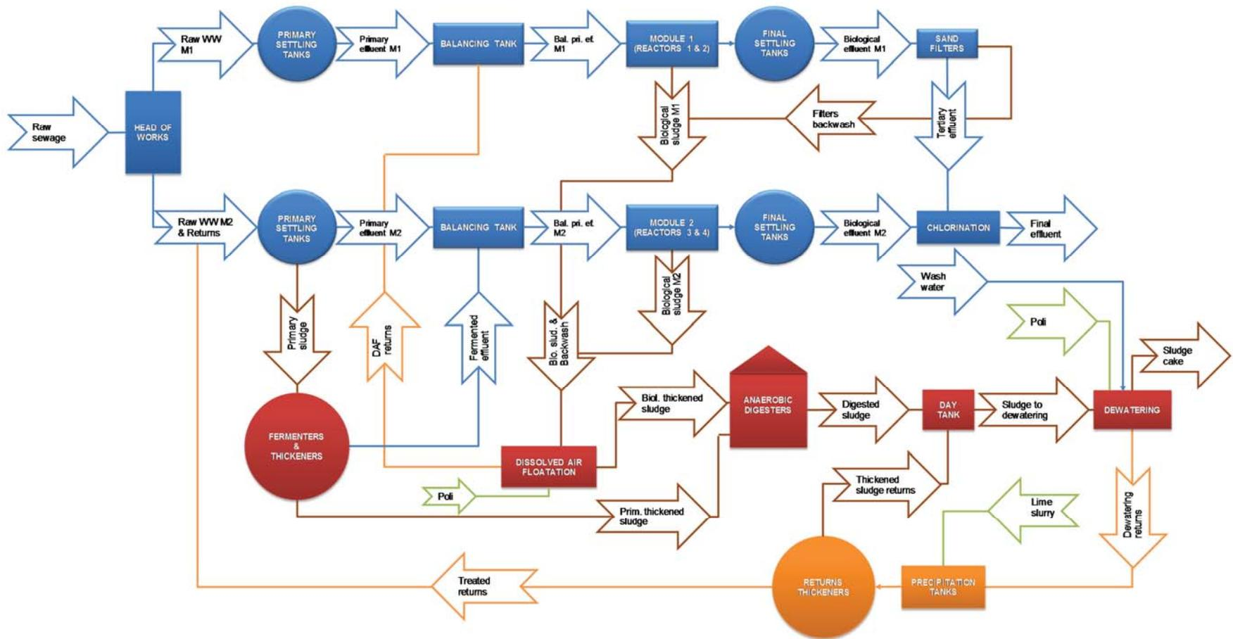
Figure 2: General process flow diagram of 'Z' WWTP
