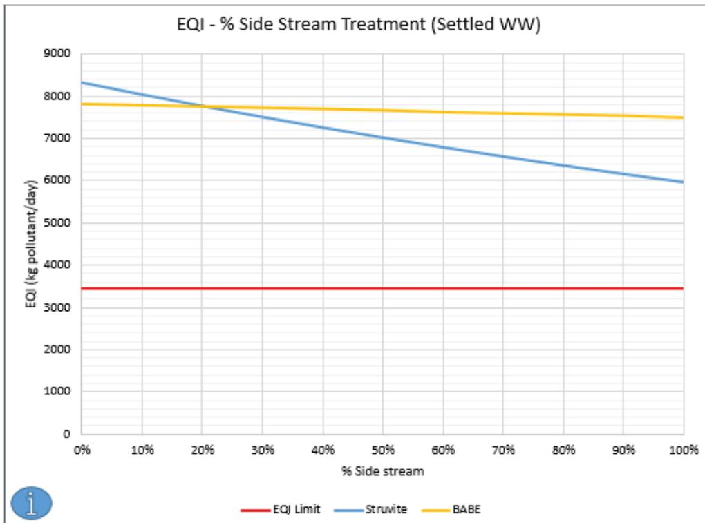
Figure 5-8: EQI variation with the percentage of dewatering liquor treated for plant B
