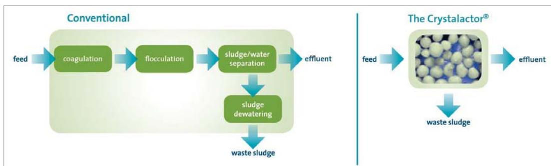
Figure 2-11: Overview of the Crystalactor® process
