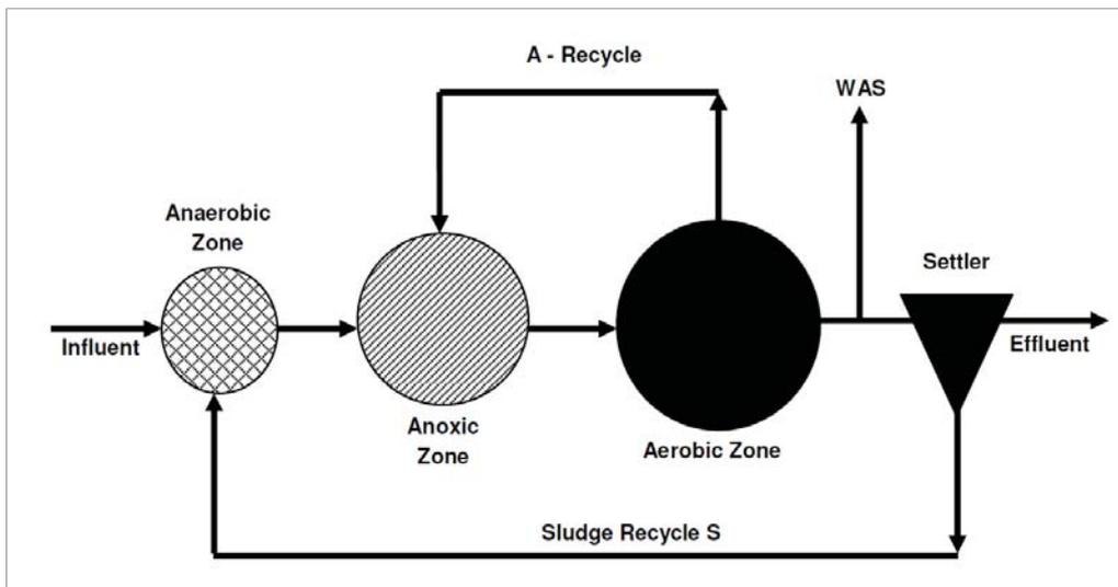
Figure 2-2: Diagrammatic layout of the Phoredox process (adapted from Ekama et al., 1984)
