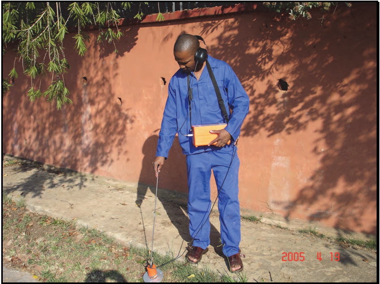
Figure 7: Leak location using sounding equipment
