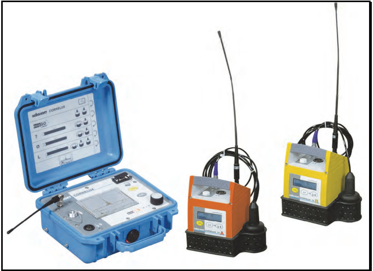
Figure 68: Leak noise correlator (courtesy Seba)
