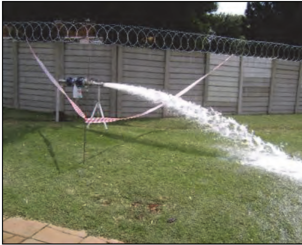
Figure 127: Typical drawdown test
