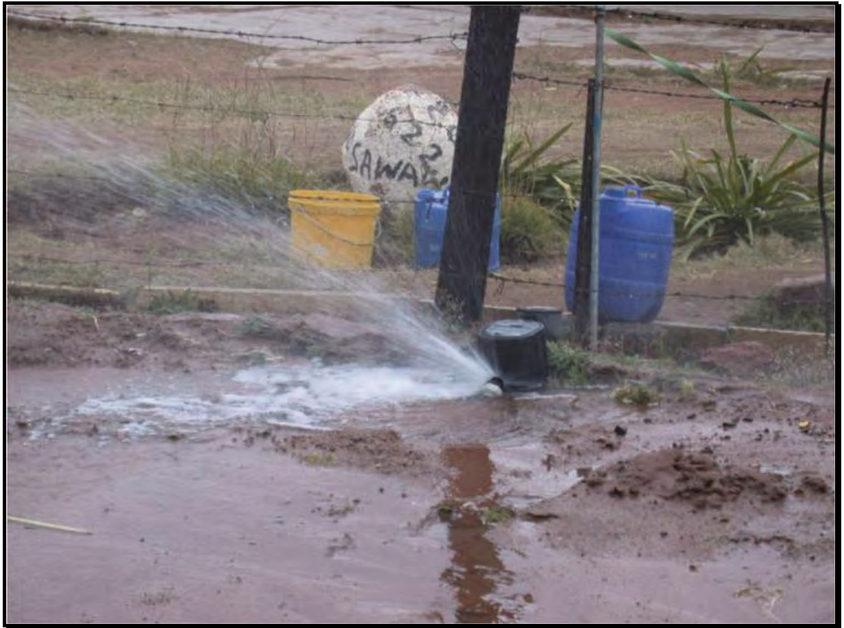
Figure 58: Small connection leak on 25mm-diameter uPVC pipe at \pm 50\text{m} pressure
