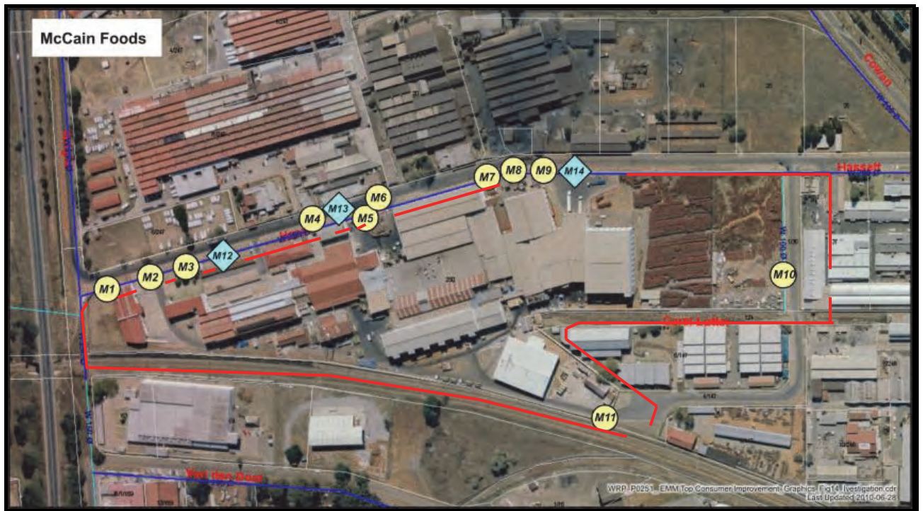
Figure 126: Illustration of Metered and un-metered connections to a single property
