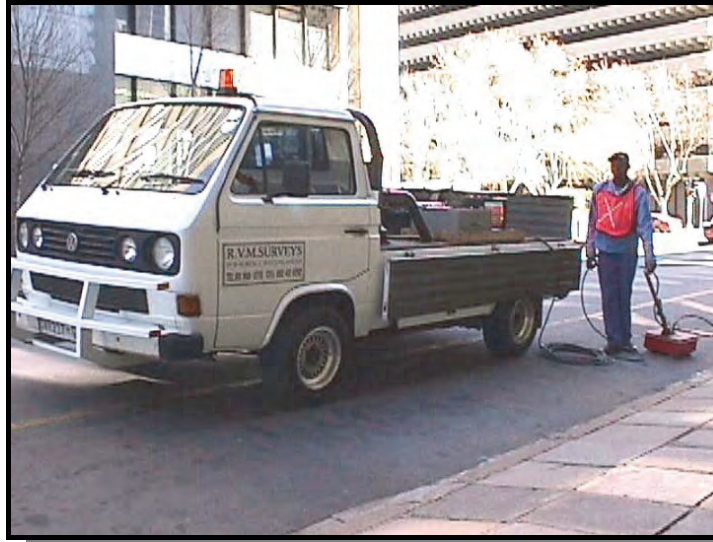
Figure 72: Ground Penetrating Radar
