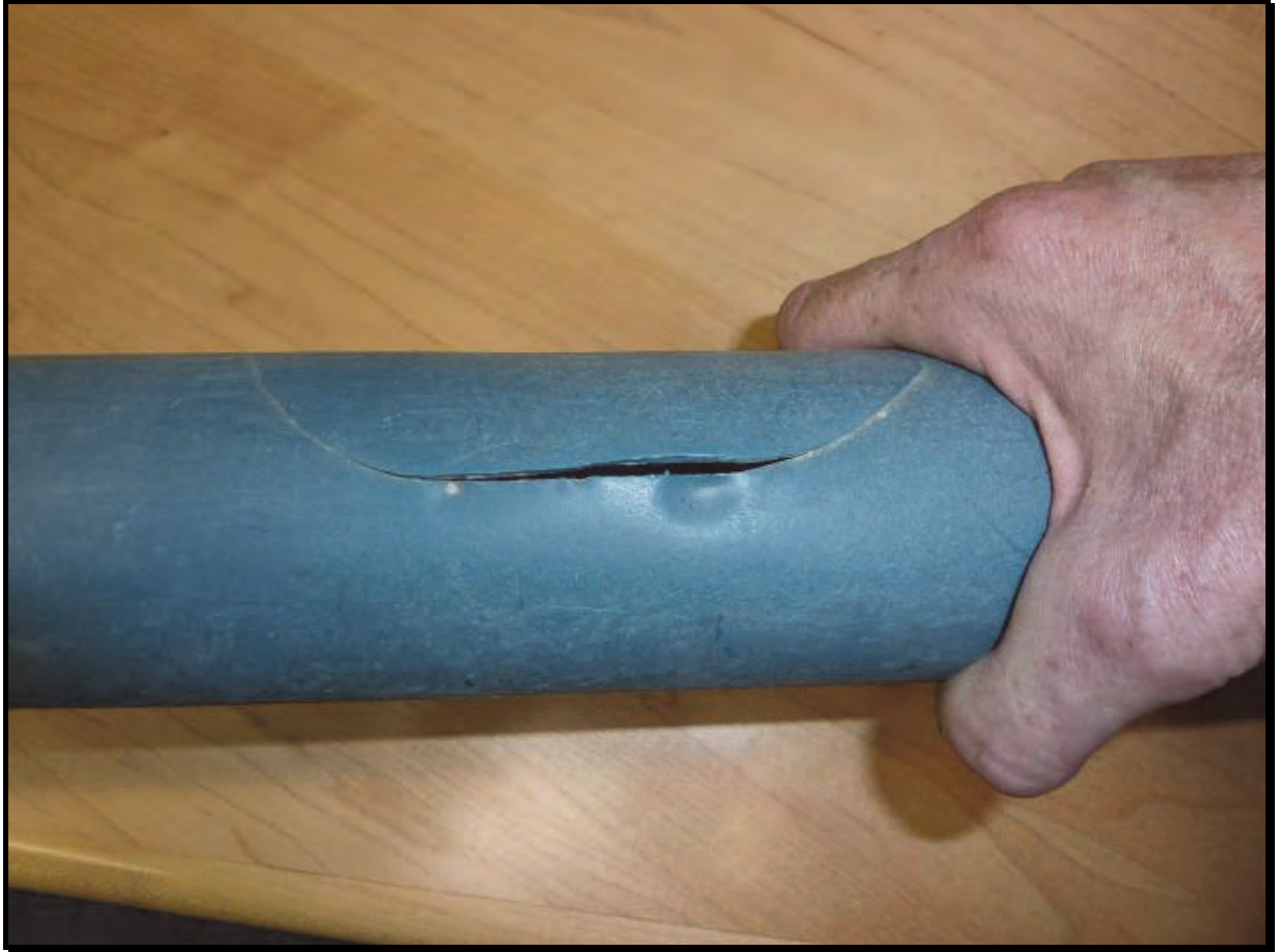
Figure 60: Leak on 63mm-diameter pipe that resulted in a R3.5 million loss
