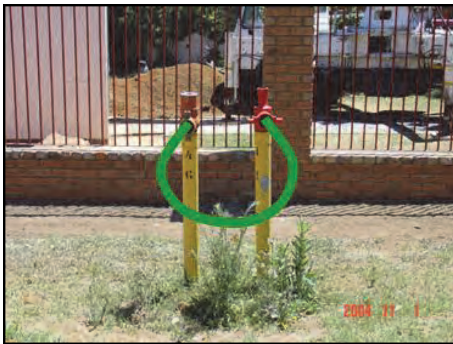
Figure 182: Approach used to identify cross boundary connections
