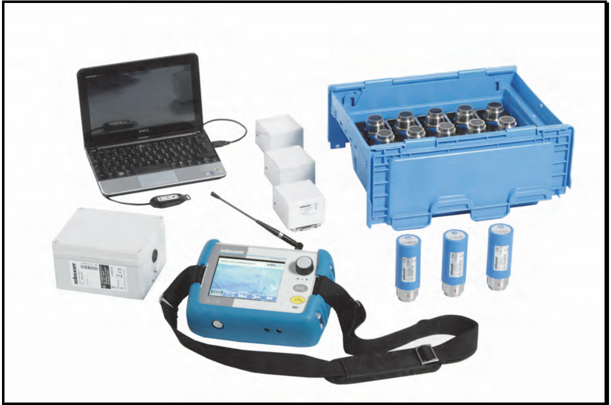
Figure 75: Typical set of Noise Loggers
