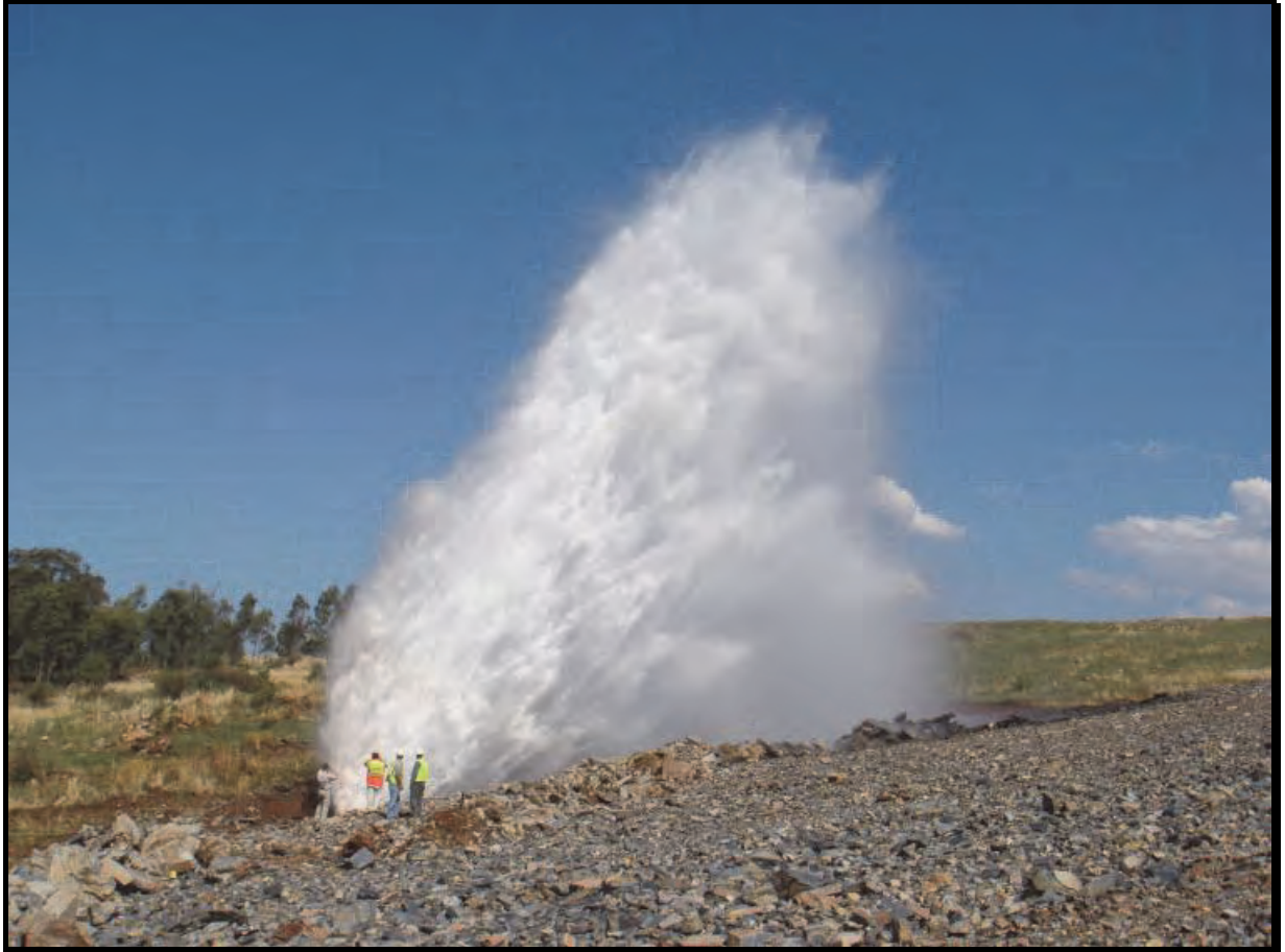
Figure 55: Leak on 600mm-diameter main at pressure of 230m (courtesy N Meyer)
