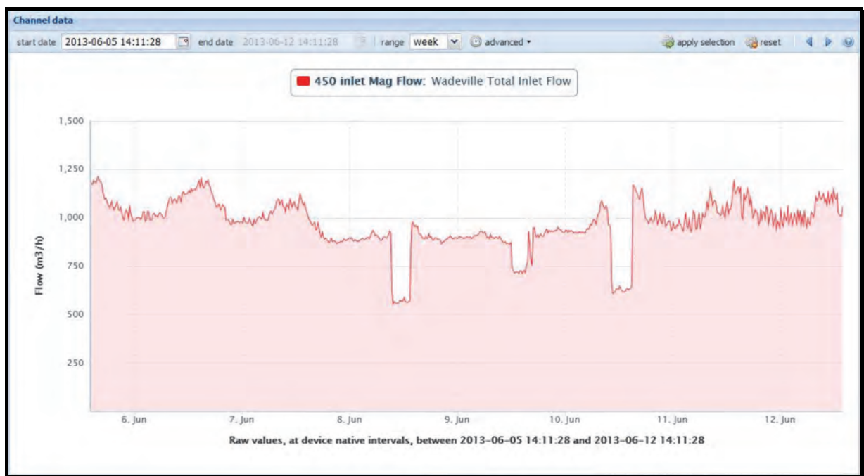
Figure 71: Typical "shut-off" for industrial consumer
