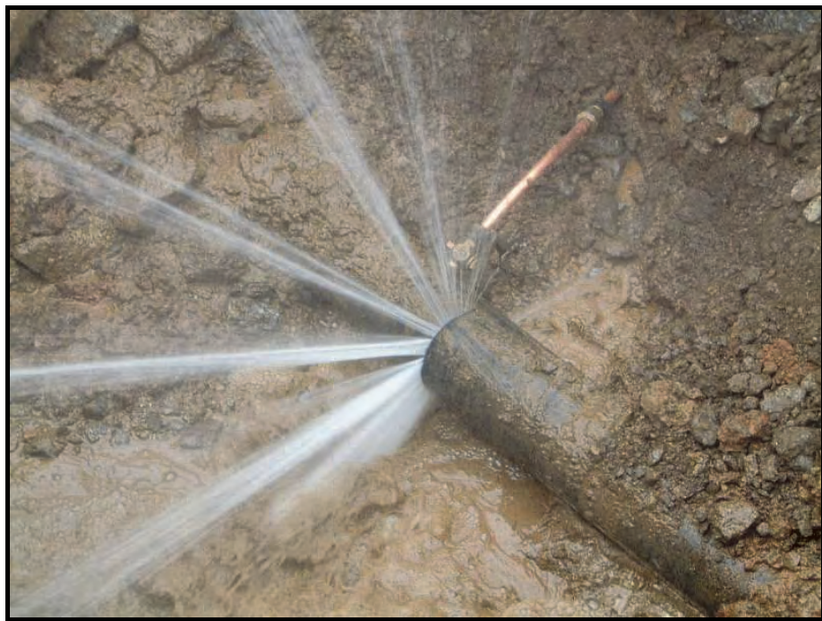
Figure 11: Underground leak running at high pressure (Ken Brothers)
