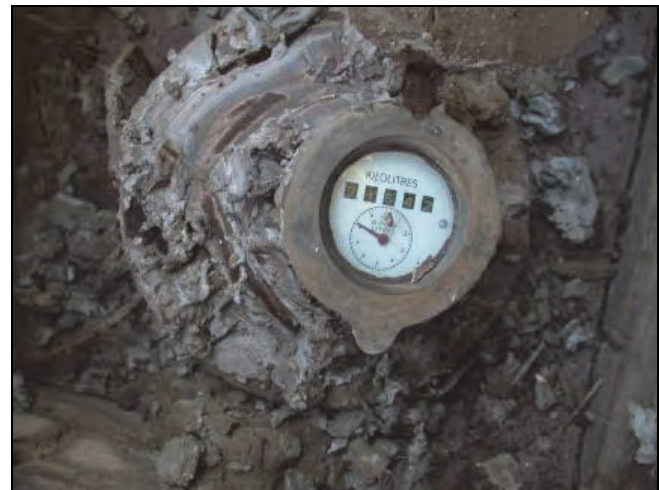
Figure 123: Non-functional and old meter
