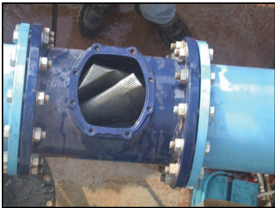
Figure 42: Damaged strainer due to small hole diameter and very high flows
