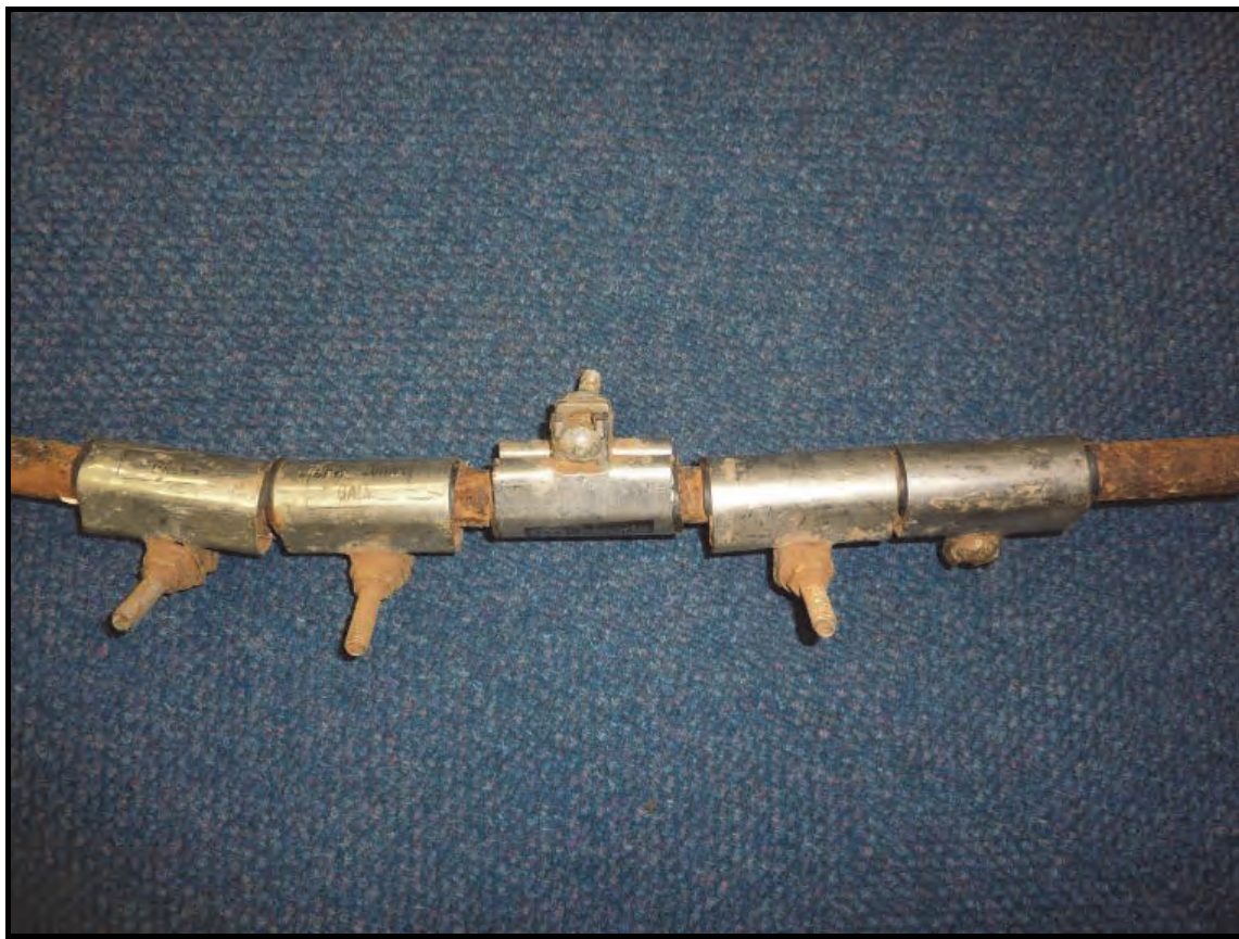
Figure 18: A case where pipe replacement is clearly appropriate
