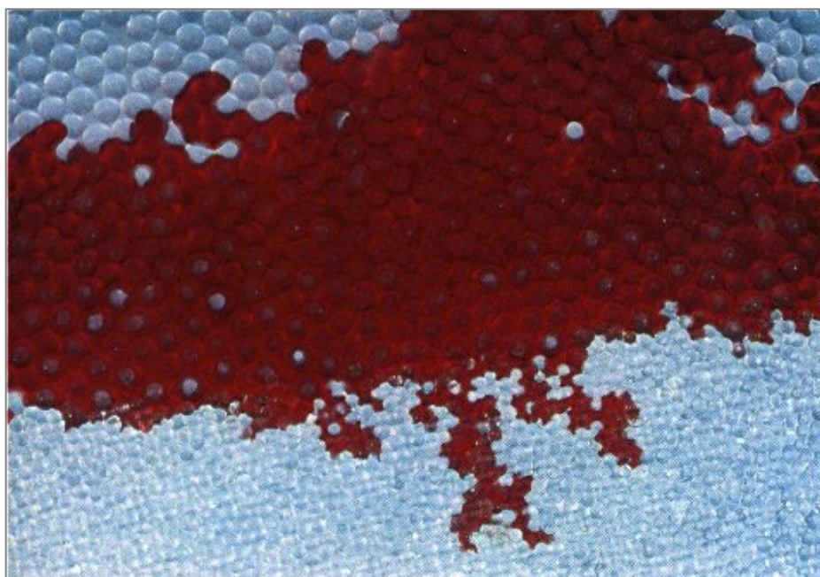
Figure 14: Example of a two-layer bead medium, initially saturated with water. Entry of smaller pore space by DNAPL only after sufficient pressure as result from pool height
