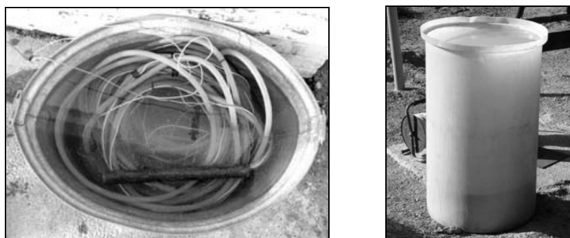
Figure 4.8. Pump and pipe disinfection containers for shallow wellpoints (left) and deeper boreholes (right).
