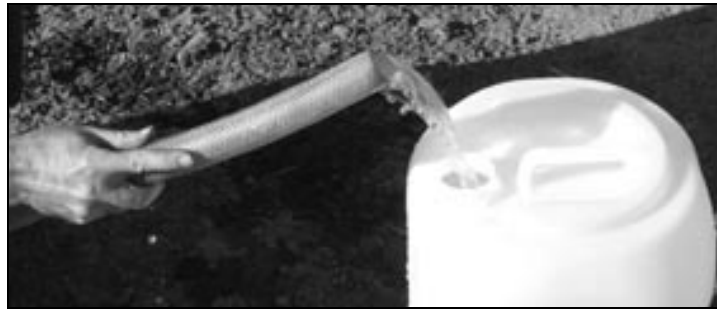
Figure 4.10. Correct sample collection procedure (end of pipe not touching the sample bottle).
