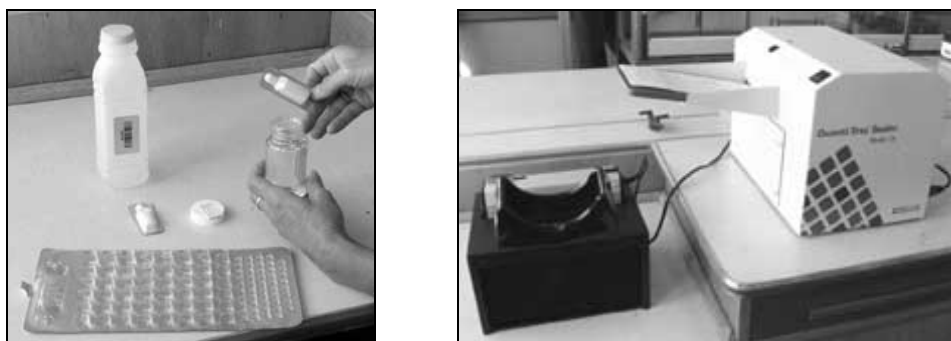
Figure 4.12: Colilert-18® Quanti-Tray (left) and Quanti-Tray sealer (right) used to detect E. coli .
