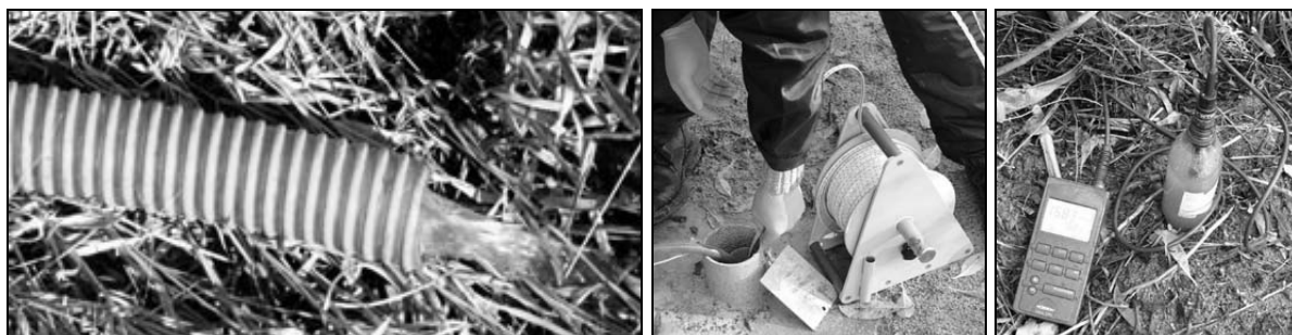
Figure 4.9. Purging (left), water level monitoring (middle) and monitoring of electrical conductivity (right).
