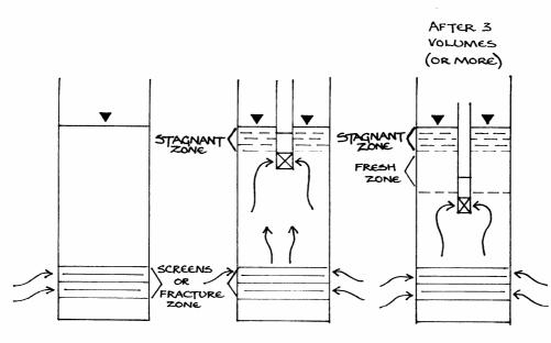
EXISTING BORE HOLE WITH SCREENS, OR OPEN HOLE WITH FRACTURED ROCK
