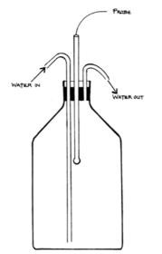
Figure 15.2. Sketch of improvised flow-through cell. The outlet tube should not protrude through the stopper into the bottle to ensure that all bubbles can readily be removed from the cell.
