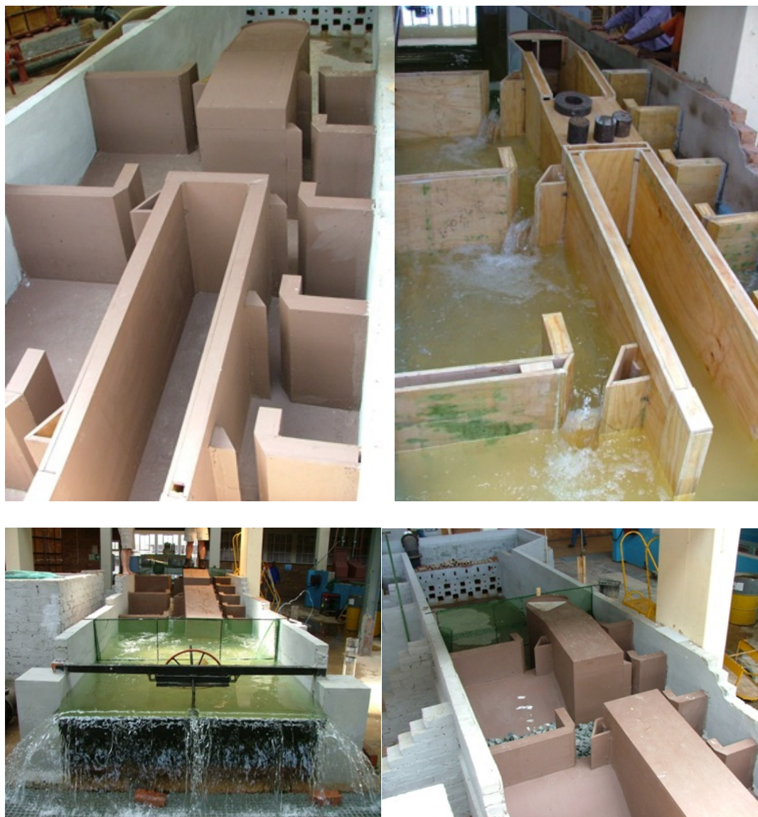
Plate 9-1: Various views of the full-scale Twin Channel Vertical Slot fishway model.
