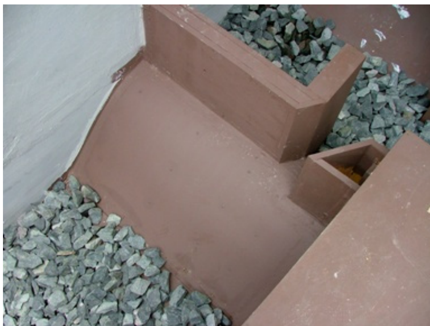
Plate 9-2: Sloping sills and substrate incorporated into a modified design.
