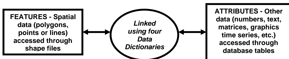
Figure 2.1 Basic data access design in SPATSIM
