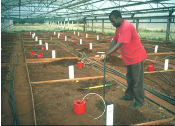
Photo 2.1 (left) The rainout shelter at the Hatfield experimental site. A hole is being augered for an electronic detector (foreground)
