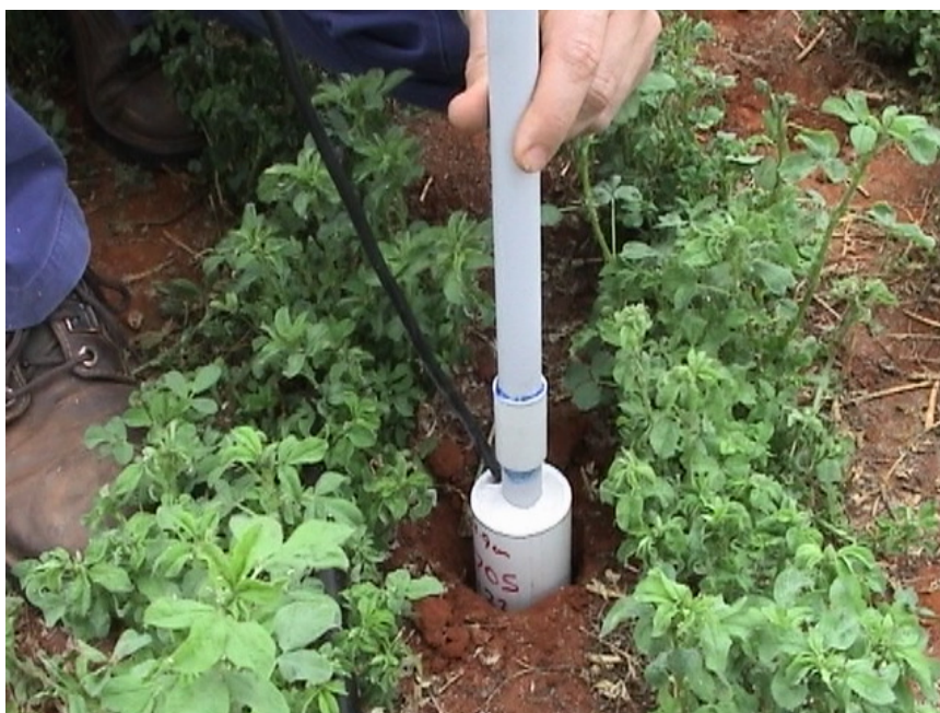
Photo 2.8 Installation of the LongStop at Hatfield. The hole above the detector can be sealed, so the response is not affected by soil disturbance
