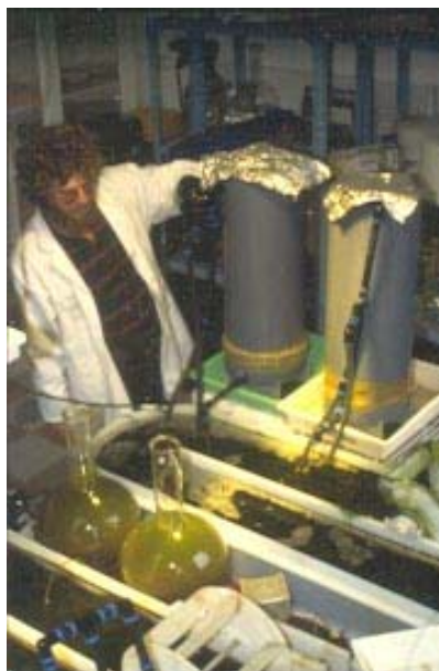
Figure 3.1 Oleg Shipin examines HRAP components of the laboratory bench-scale pilot plant used to investigate IAPS-based treatment of abattoir wastewaters..
