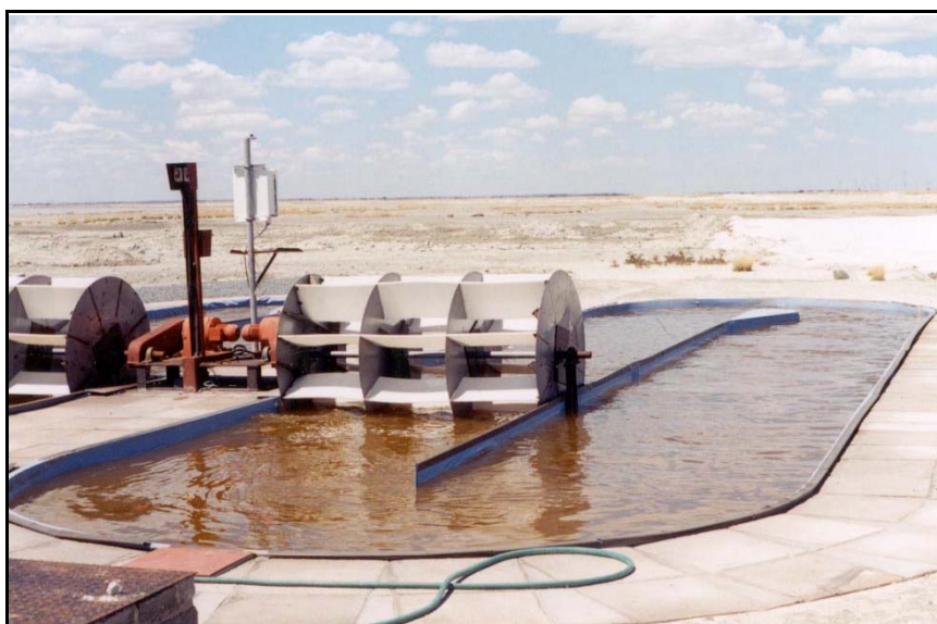
Figure A3.3. The Dunaliella -HRAP pilot plant treating saline carbonate brines at Botswana Ash Co. Sua Pan, Botswana.
