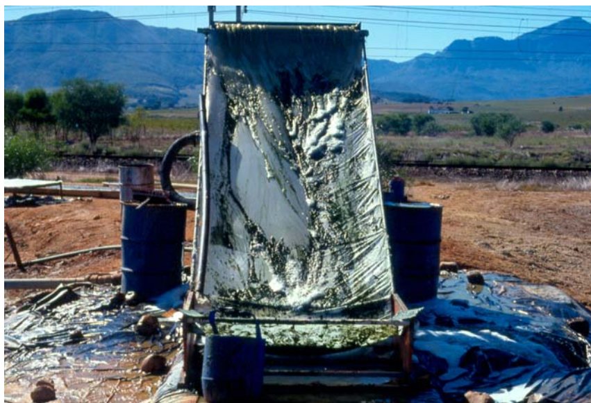
Figure 7.1 Screen harvester and drying racks used for the recovery of Spirulina biomass from the WSP at Wellington
