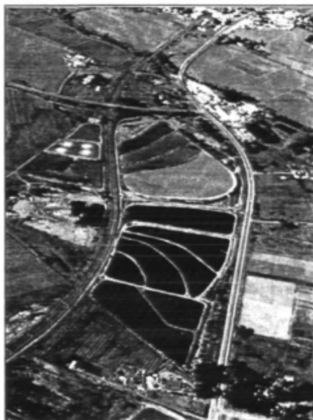
**Figure 1.1.** The Waste Stabilisation Pond evaporative disposal system treating tannery wastewaters at the Mossop-Western Leathers Co. Wellington. This unit was used as a model for the investigations on ponding systems reported in this study.
