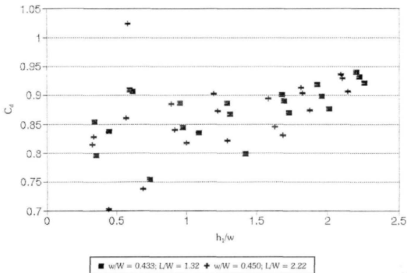
Figure 5.5 The effect of parameter L on the calibration coefficient  $C_d$
