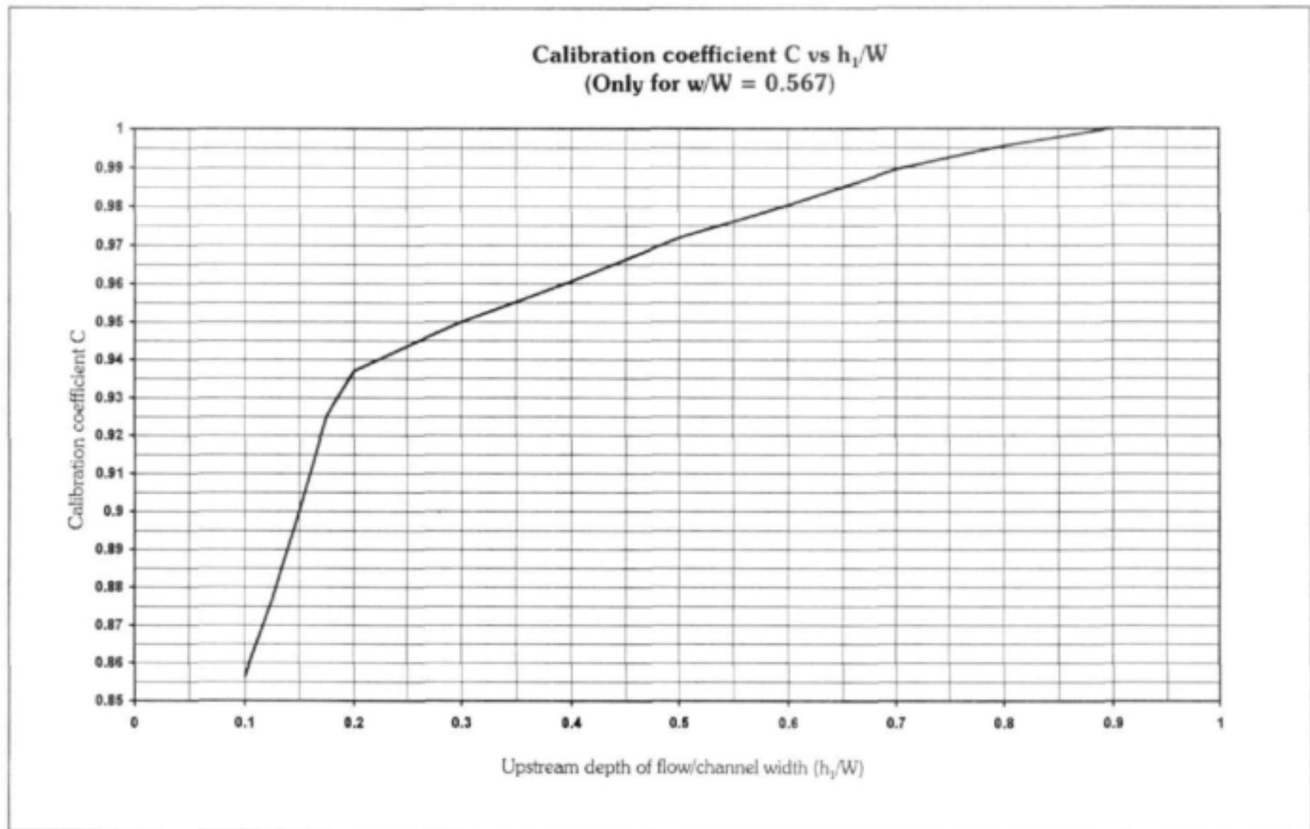
**Figure C.1: Calibration coefficient C vs.  $h_1/W$  for  $w/W = 0.567$**
