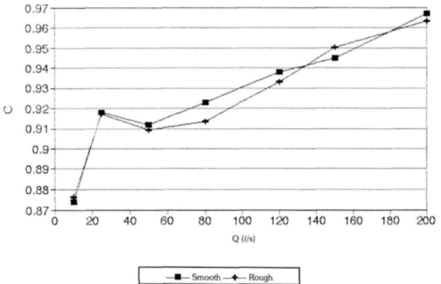
Figure 5B.1 Effect of flume roughness on calibration coefficient C
