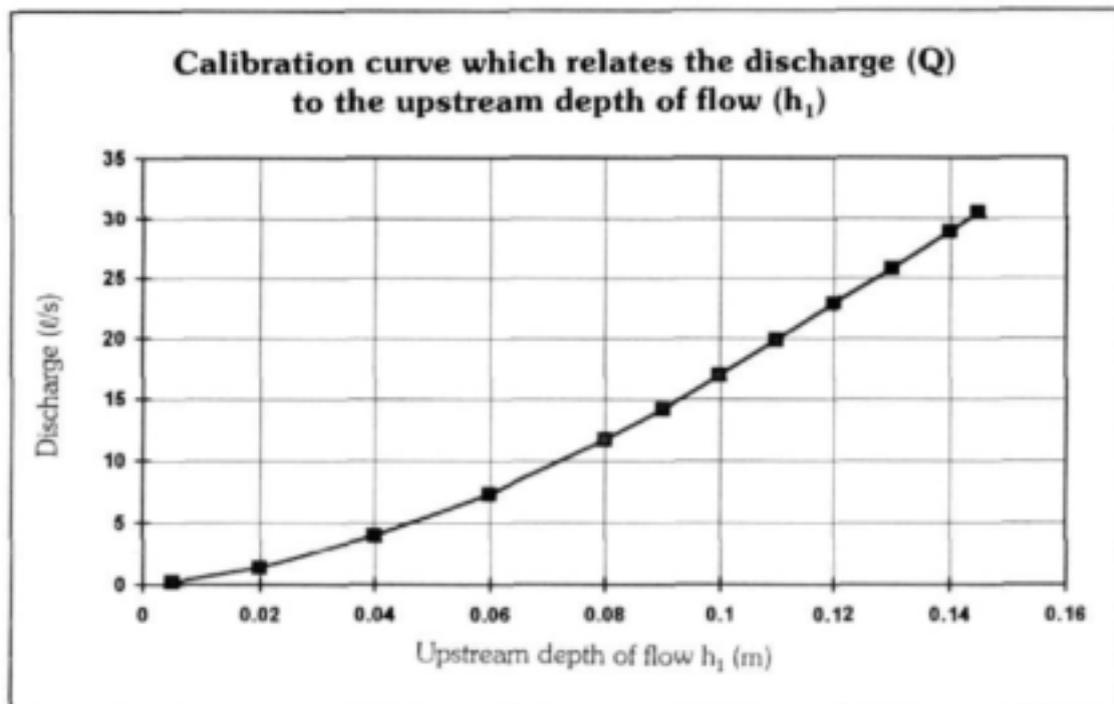
**Figure B.1 Unique relationship between discharge (Q) and upstream depth of flow ( $h_1$ )**
