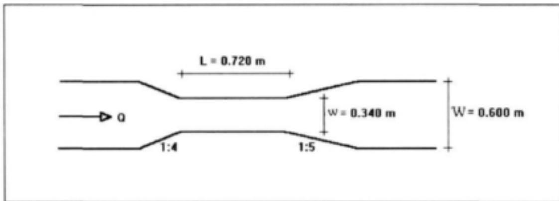
**Figure. 8.1 Standard measuring flume dimensions**
