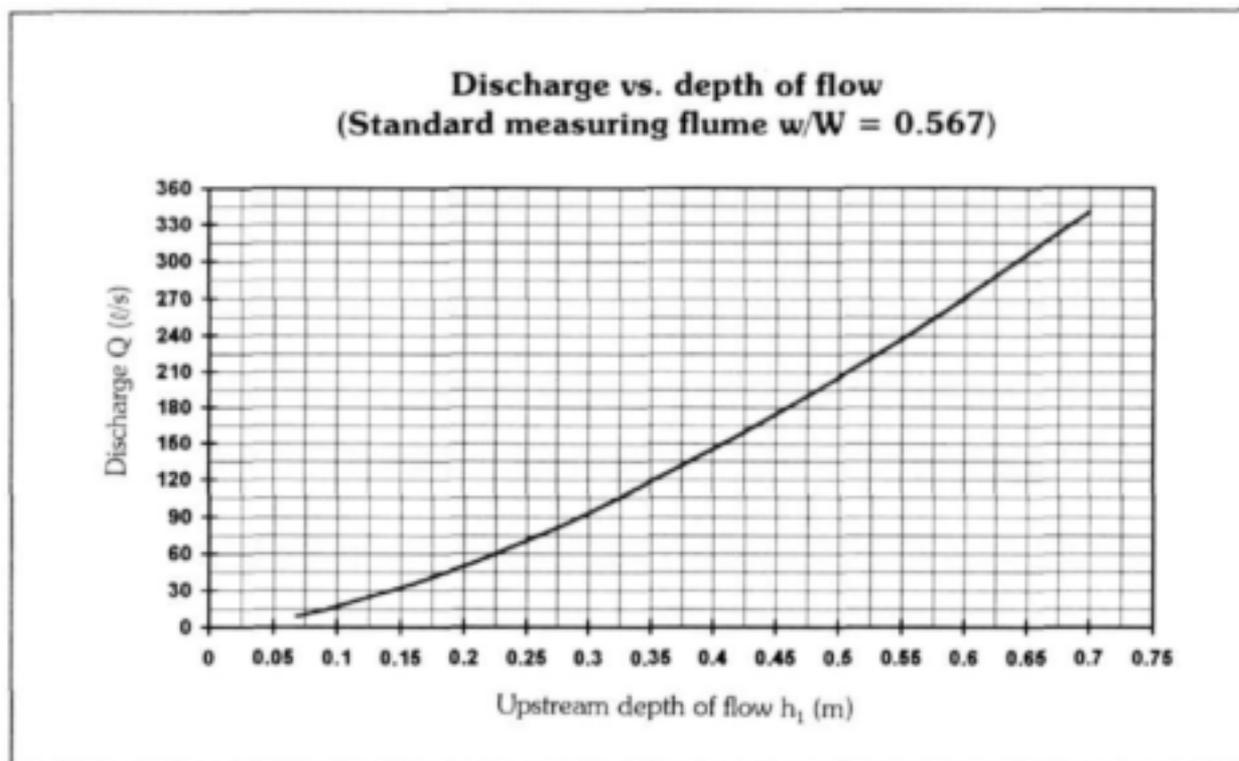
**Figure 8.2 Discharge vs. depth of flow (only for standard measuring flumes)**
