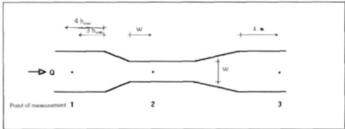
**Figure 2.2 Points of measurement in the measuring flume**
