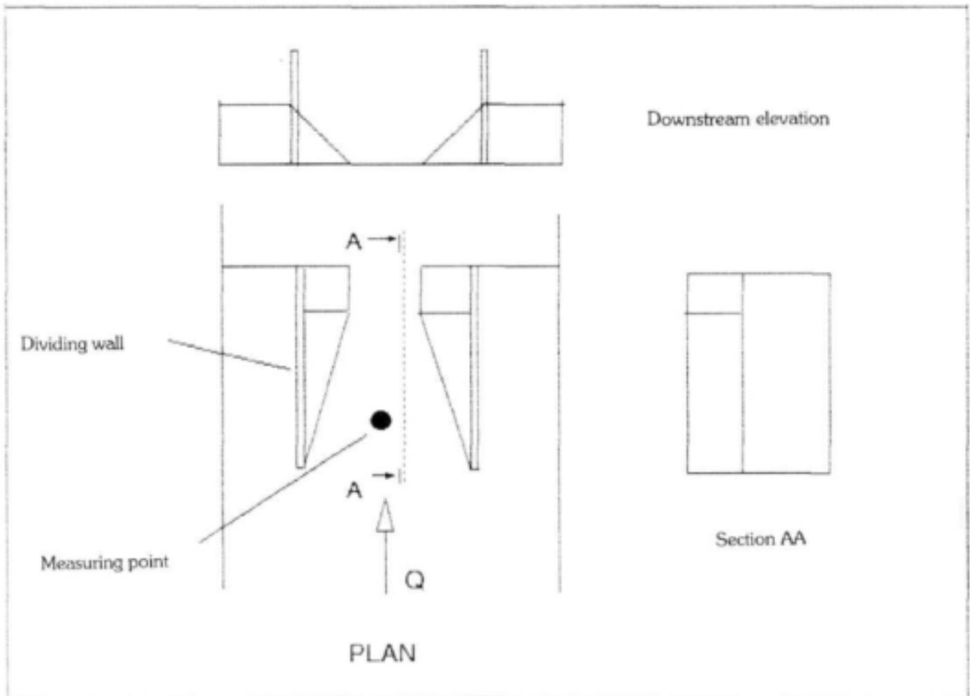
**Figure 7.2 Typical new measuring flume (sluicing flume) designed to sluice sediment**
