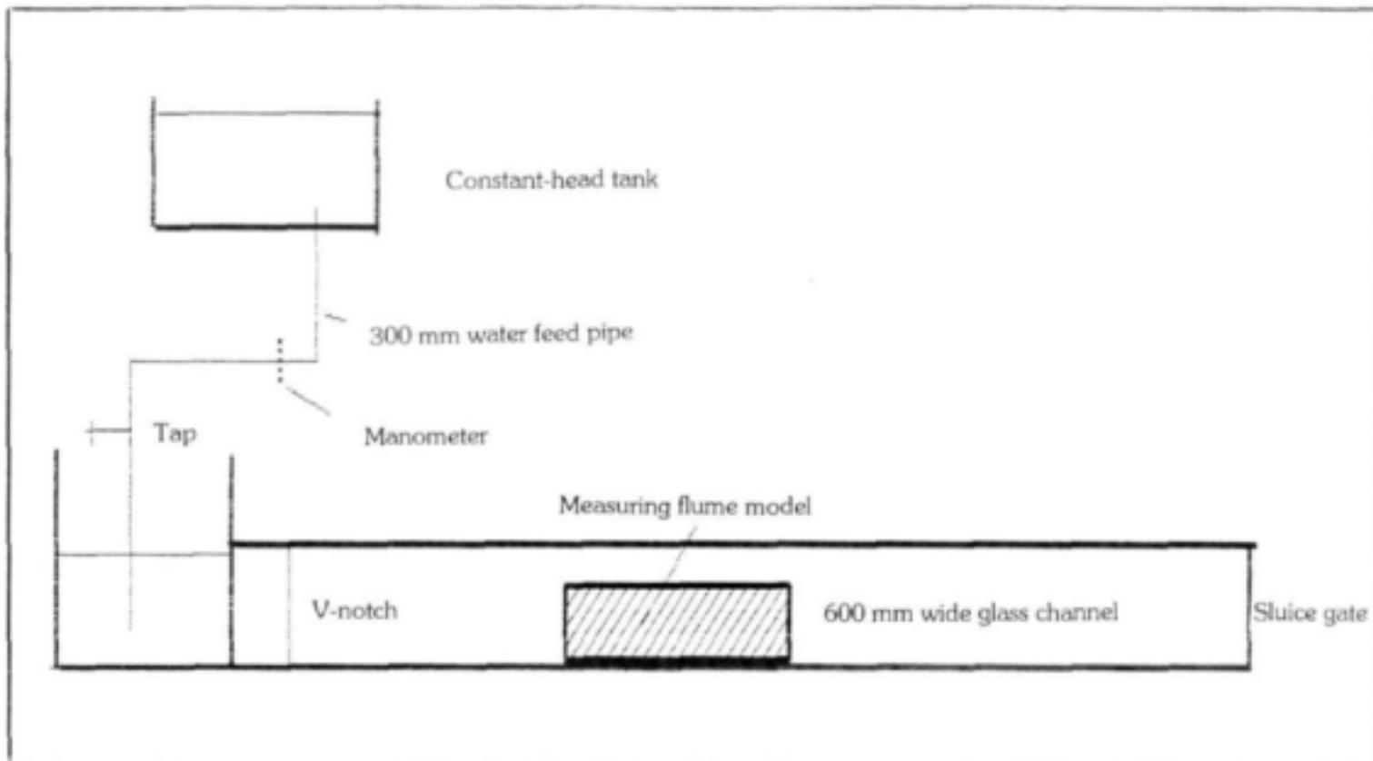
Figure 3.1 Schematic model layout in the laboratory
