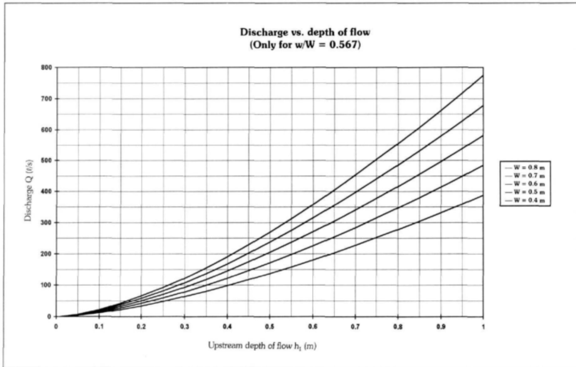
**Figure C.4: Discharge vs. depth of flow for  $w/W = 0.567$  and  $0 \leq h_1 \leq 1$  m**
