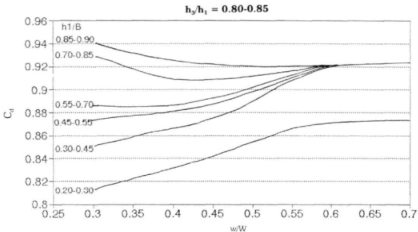
Figure 5.3 Determining calibration coefficient  $C_d$  ( $h_2/h_1=0.80$  to  $0.85$ )
