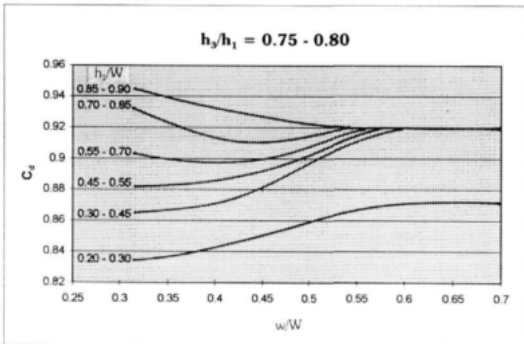
**Figure 3.2 Determination of the calibration coefficient  $C_d$  ( $0.75 < h_2/h_1 < 0.80$ )**
