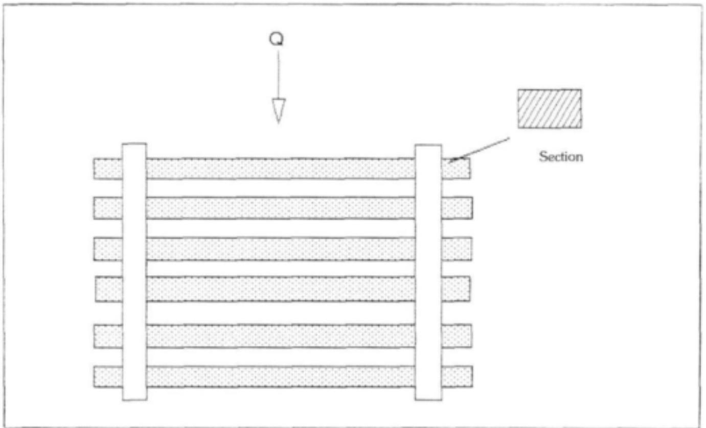
**Figure 7.1 Wooden slats to dampen surface wave action**
