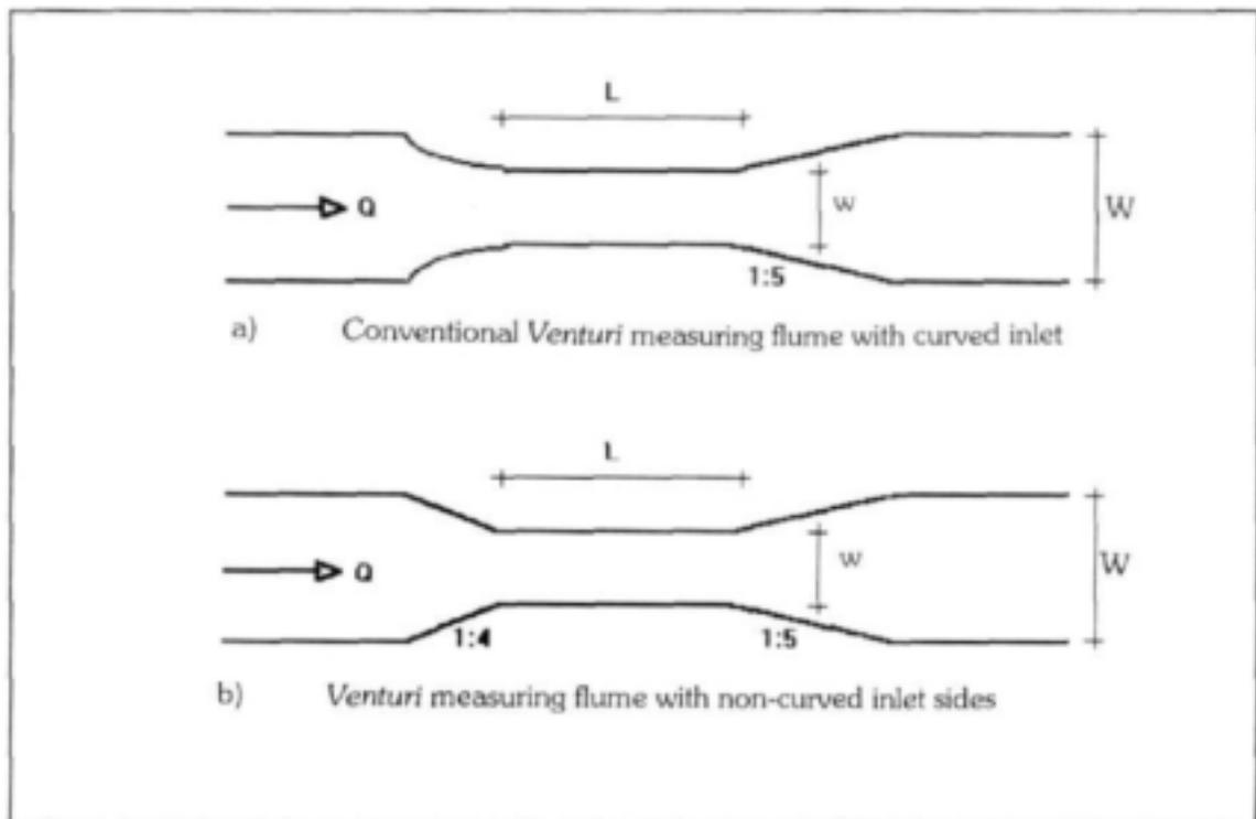
**Figure 2.1 Layout of measuring flumes**
