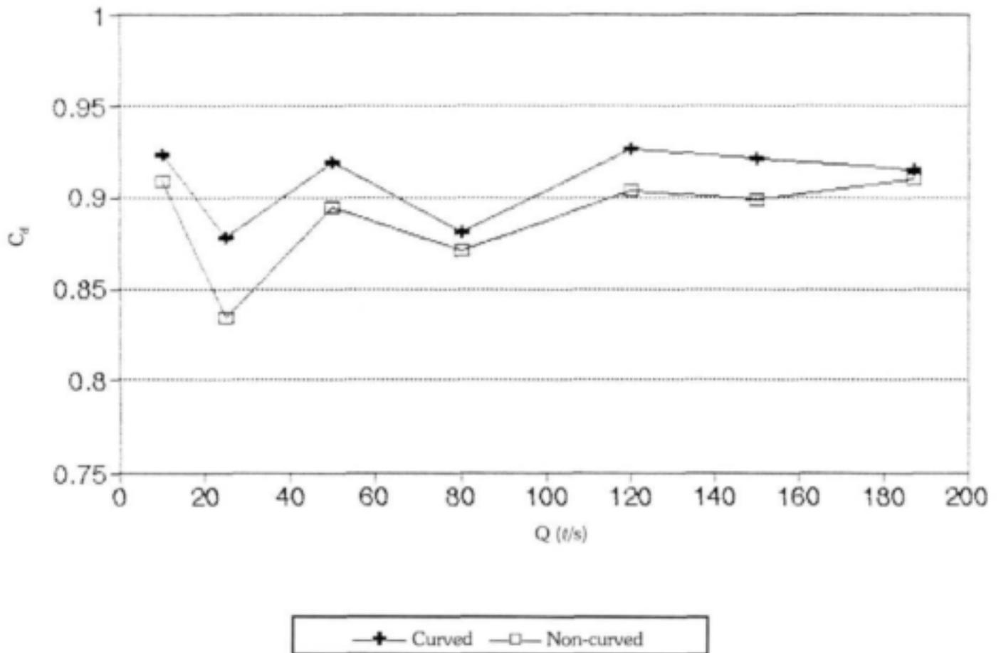
Figure 5A.2 The effect of inlet shapes on the calibration coefficient  $C_d$
