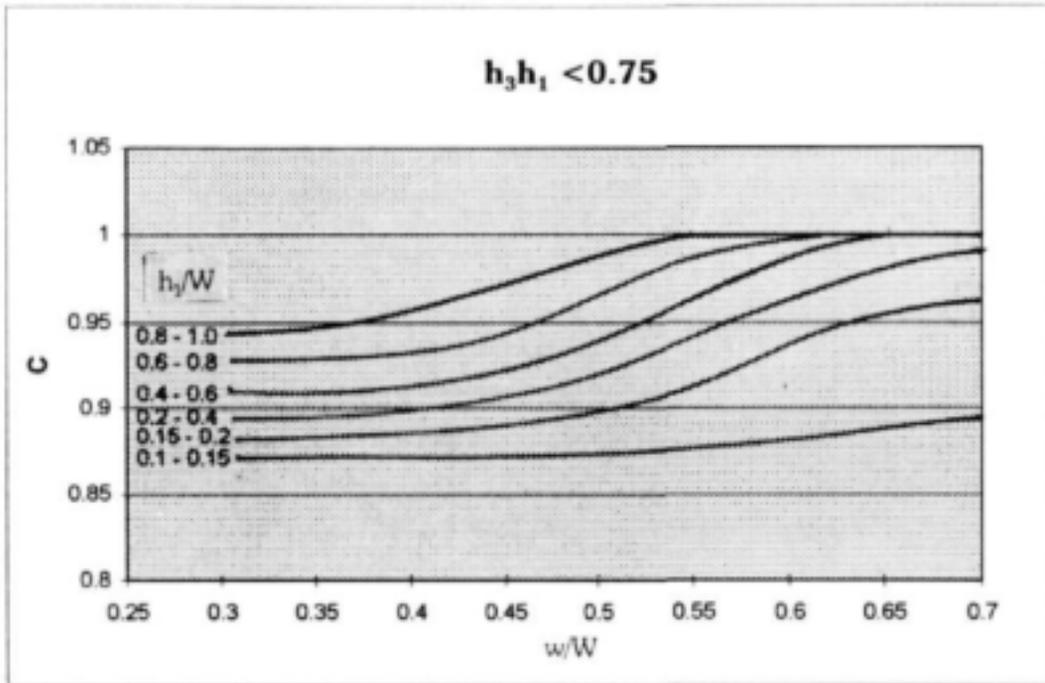
**Figure 3.1 Determination of the calibration coefficient  $C$**
