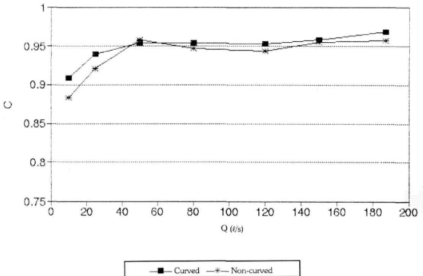
Figure 5A.1 The effect of inlet shapes on the calibration coefficient C
