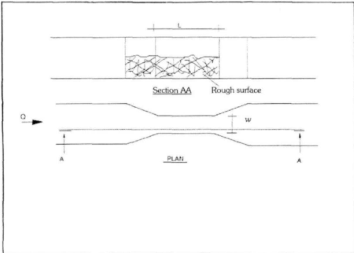
Figure 5.6 Measuring flume surface area roughened for roughness tests
