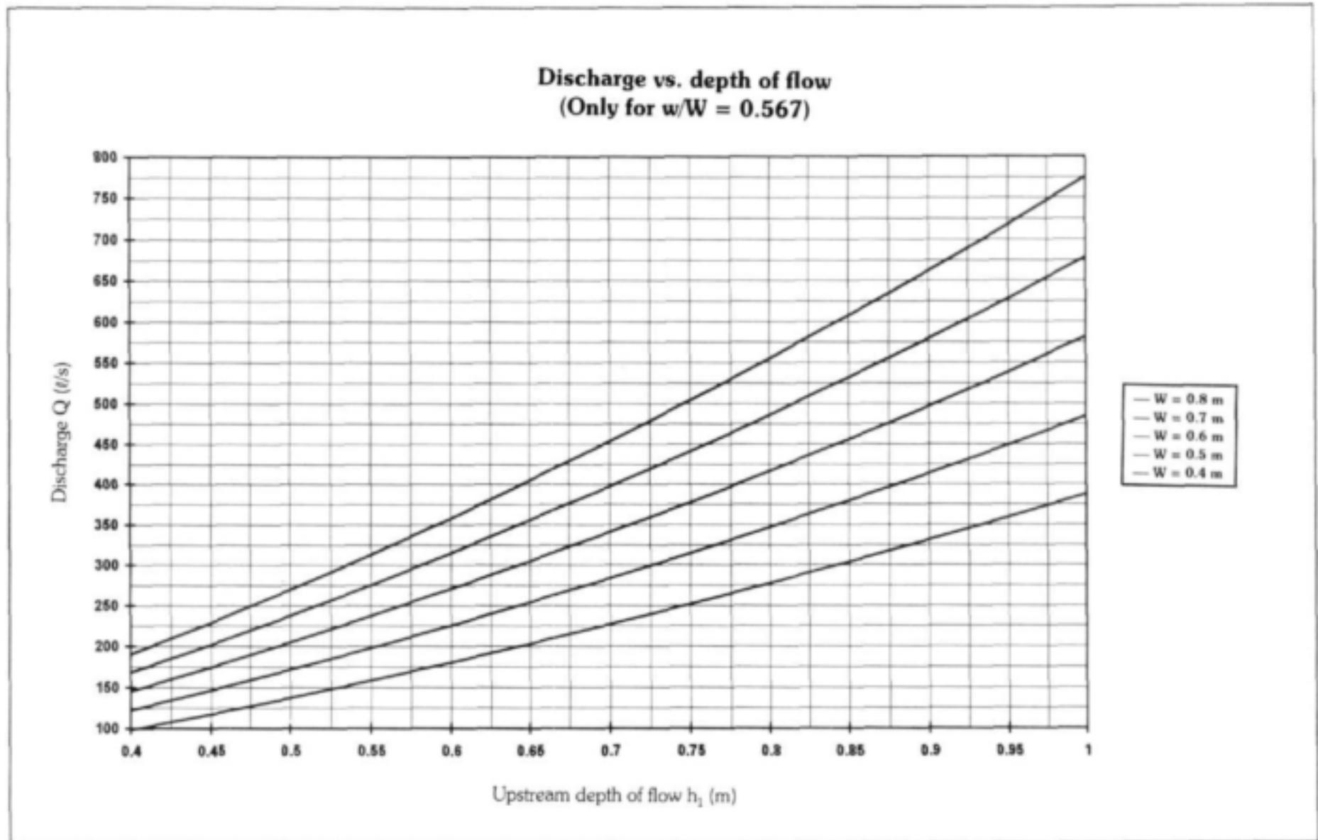
Figure C.3: Discharge vs. depth of flow for  $w/W = 0.567$  and  $0.4 \leq h_1 \leq 1$  m
