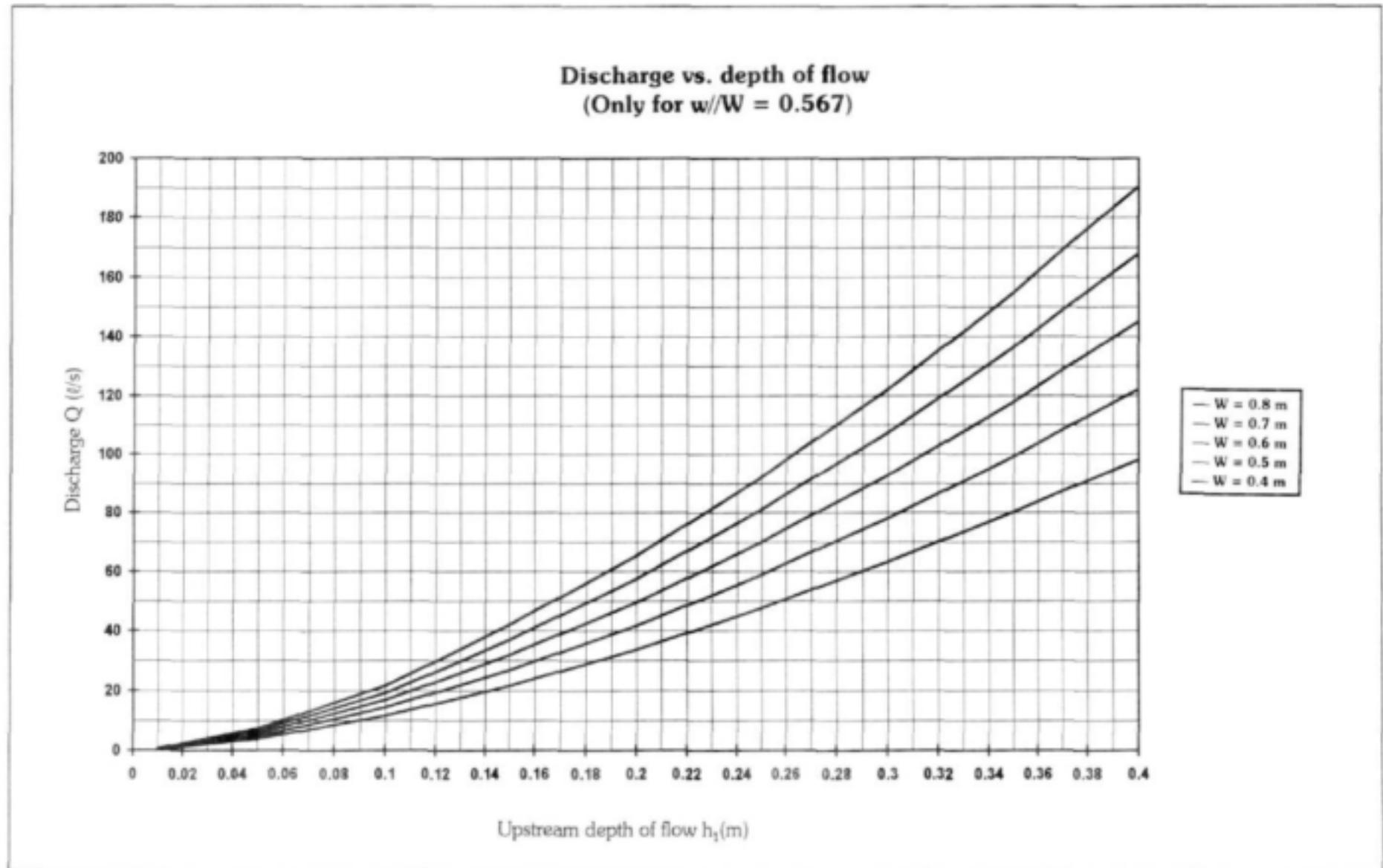
Figure C.2: Discharge vs. depth of flow for  $w/W = 0.567$  and  $0 \leq h_1 \leq 0.4$  m
