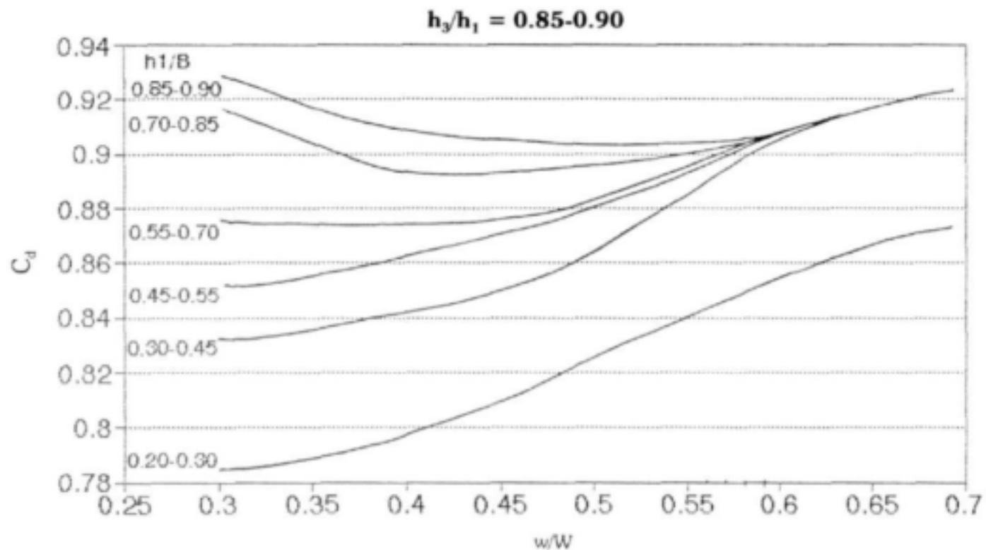
Figure 5.4 Determining calibration coefficient  $C_d$  ( $h_2/h_1=0.85$  to  $0.90$ )
