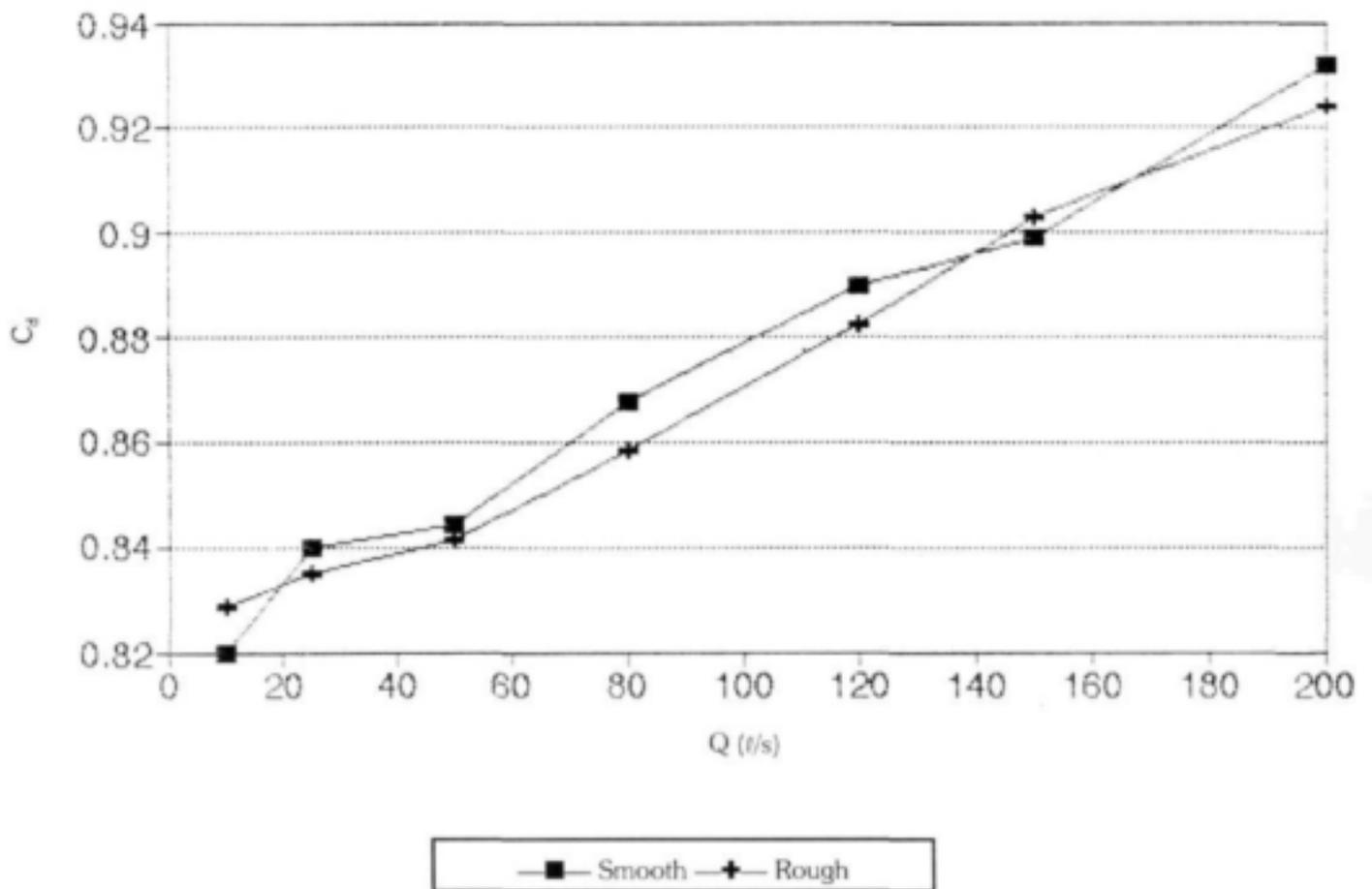
Figure 5B.2 Effect of flume roughness on the calibration coefficient  $C_d$
