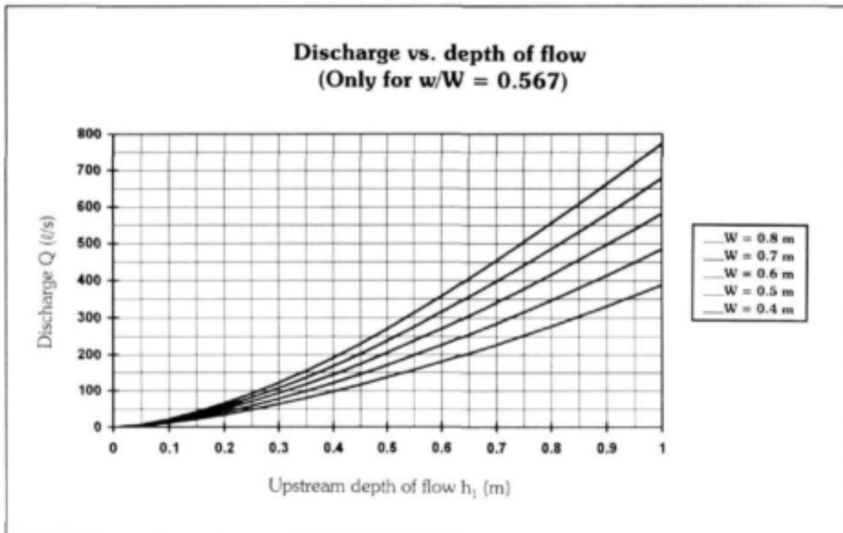
**Figure 8.4** Discharge vs. upstream depth of flow (valid for standard flumes and any up- or down-scaled versions)
