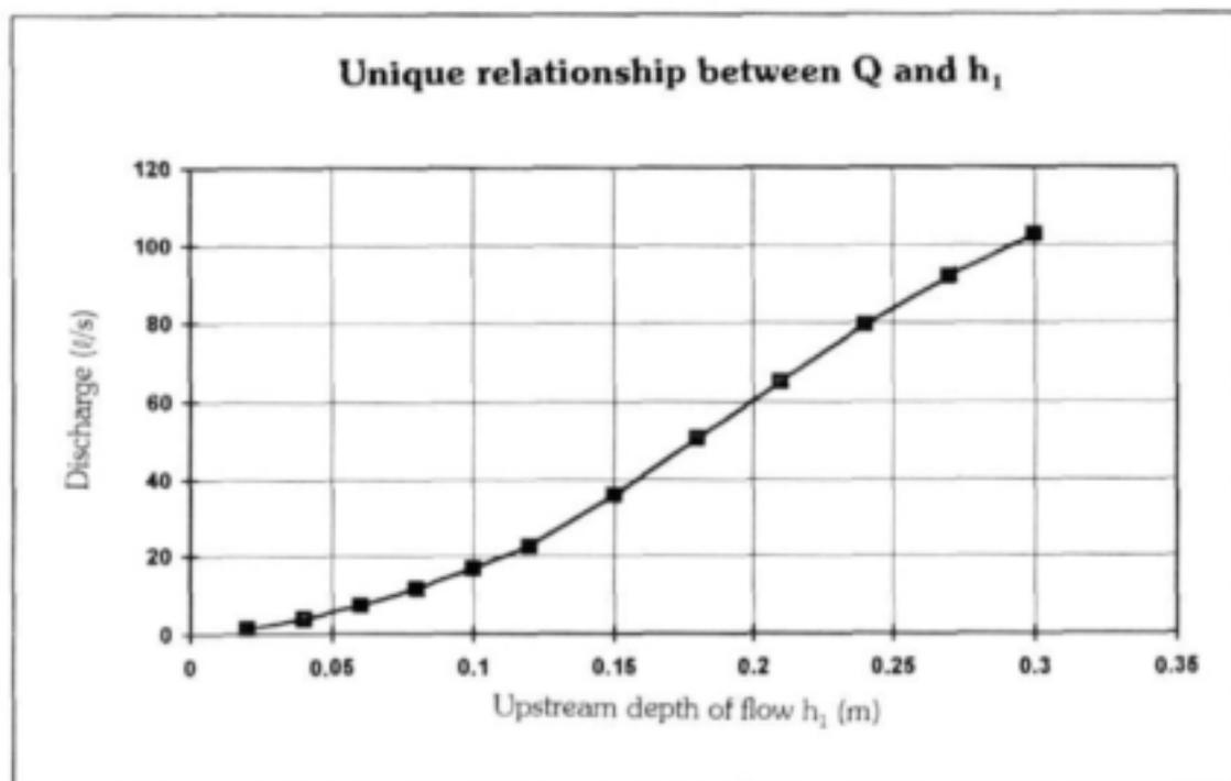
**Figure B.2 Unique relationship between discharge (Q) and the upstream depth of flow ( $h_1$ )**
