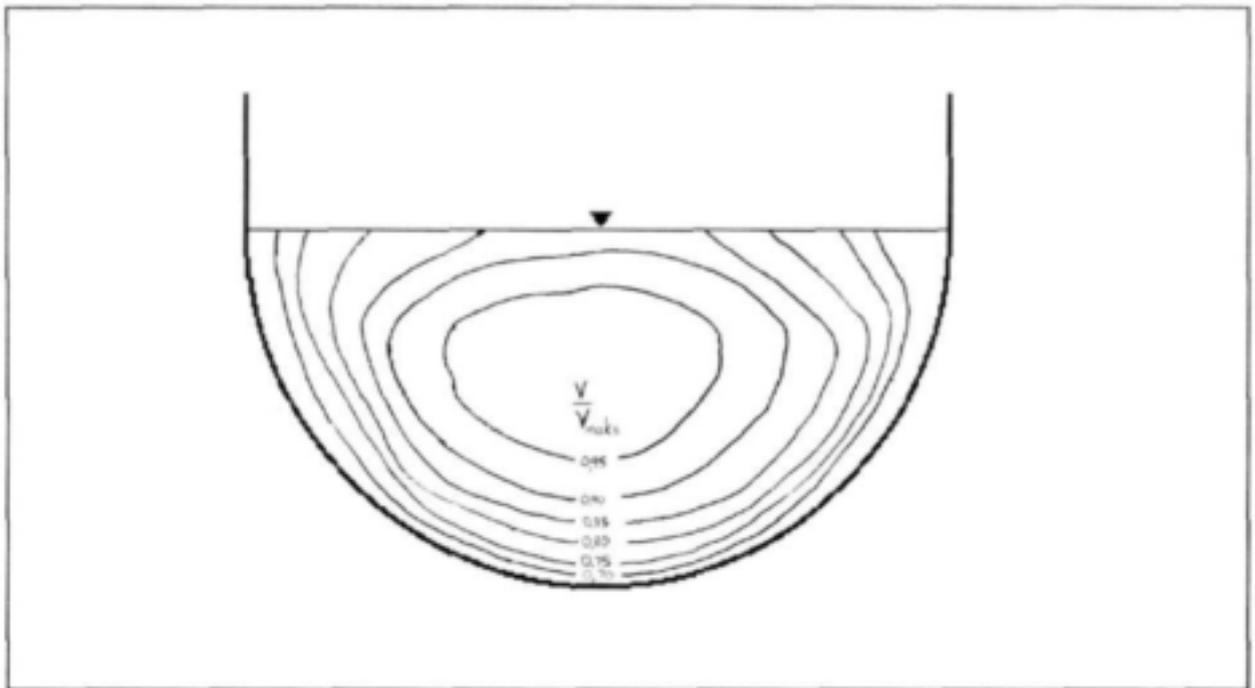
**Figure 5.2 Typical velocity contours in a cylindrical measuring channel**
