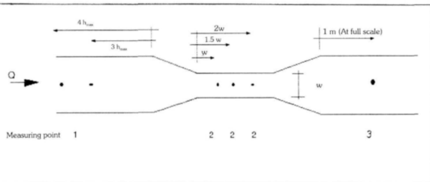
**Figure 4.1 Definition of measuring points**
