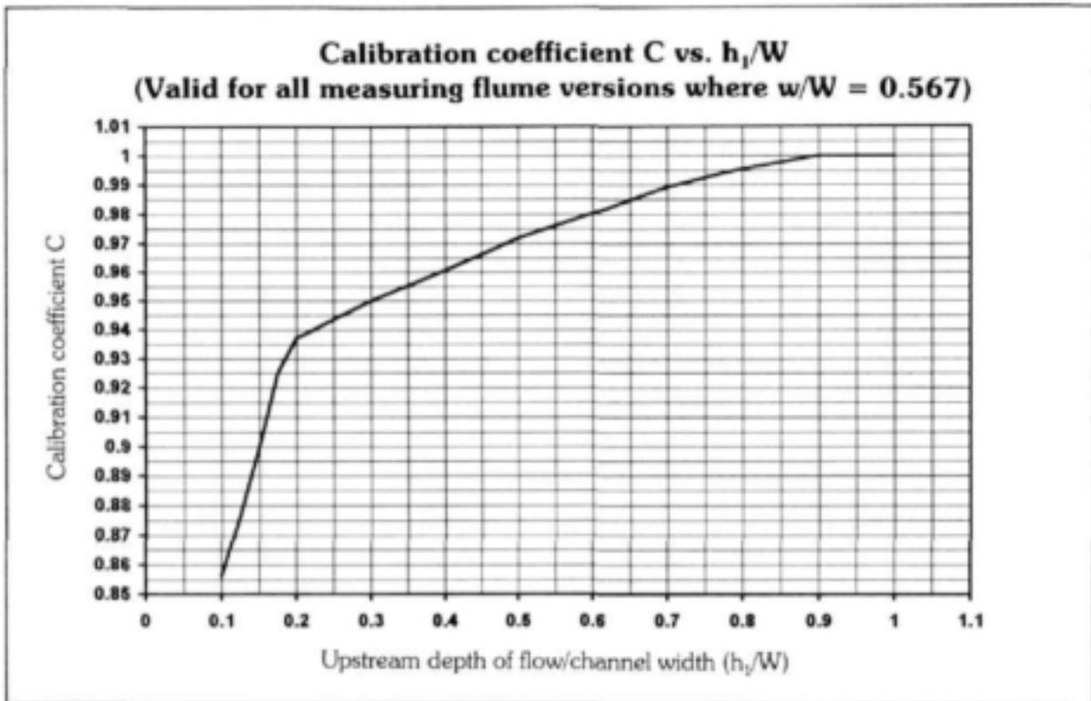
**Figure 8.3** C vs.  $h_1/W$  (valid for standard flumes and any up- or down-scaled version)
