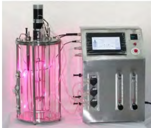
Figure 4.9 Laboratory setup for hydrogen production through photo-fermentation
