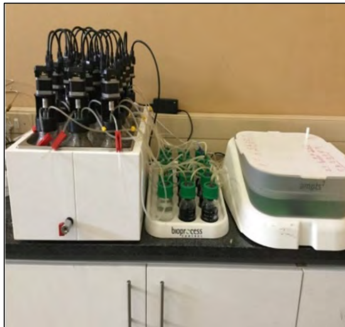
Figure 4.5 Laboratory batch reactors for conducting dark fermentation tests
