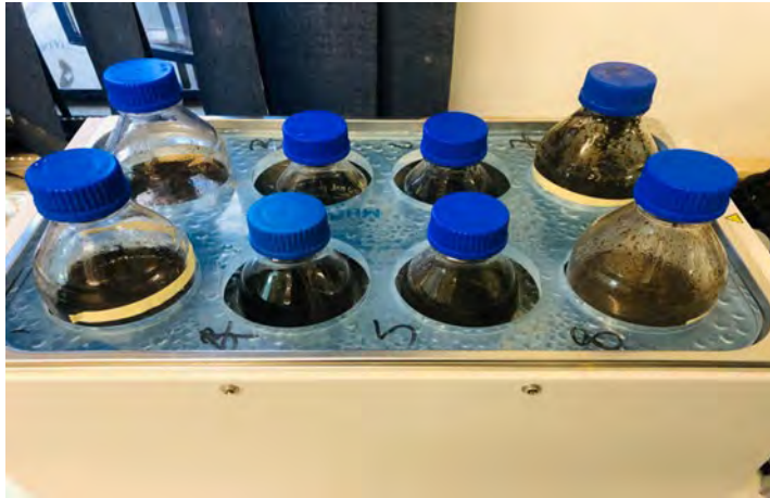
Figure 5.4 Reactor bottles containing inoculum were subjected to heat pre-treatment at 80 degrees Celsius
