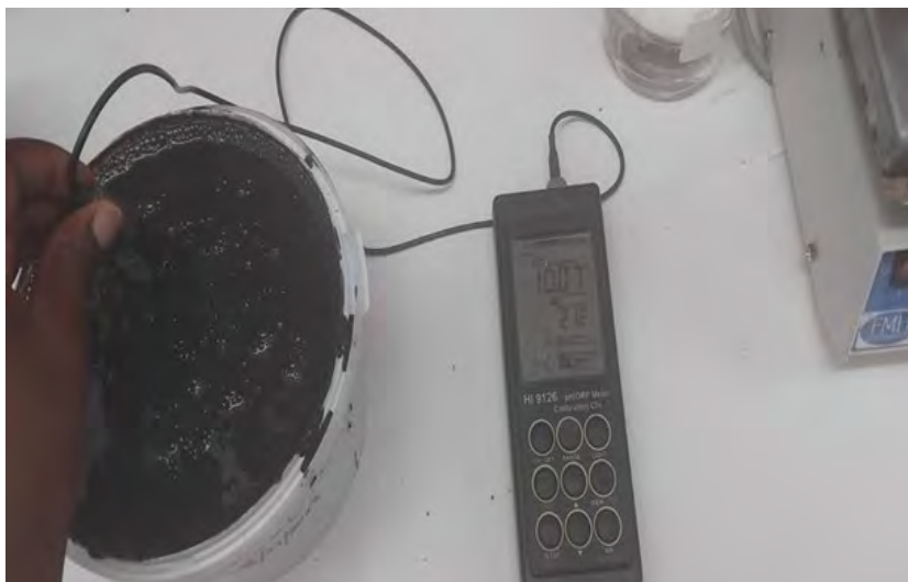
Figure 5.5 Measuring inoculum pH adjustment for alkaline pre-treatment
