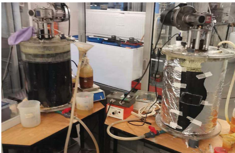
Figure 3.2: Anaerobic digesters (AD1 and AD2)
