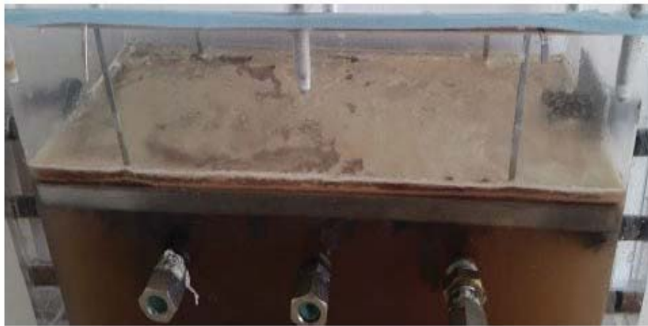
Figure 2.2: Hybrid linear flow channel reactor (HLFCR)
