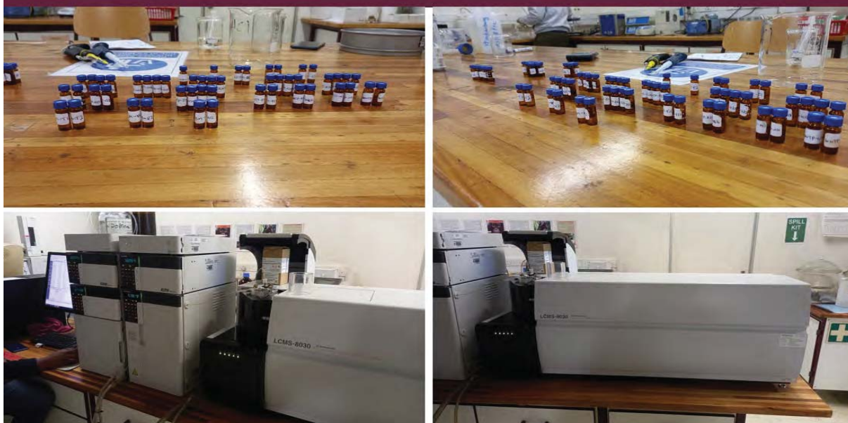
Figure 4-8: Sample vials ready for analysis run and LC-MS instrument.
