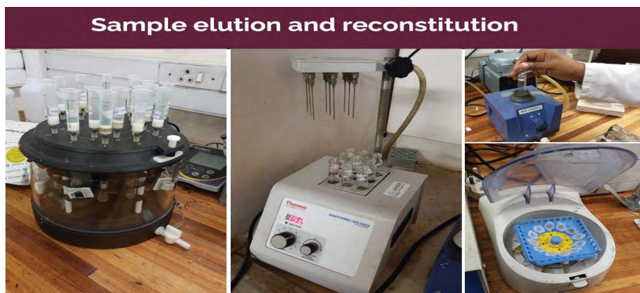
Figure 4-4: Sample elution under the force of gravity, sample concentration under nitrogen, sample shaking and centrifuging.
