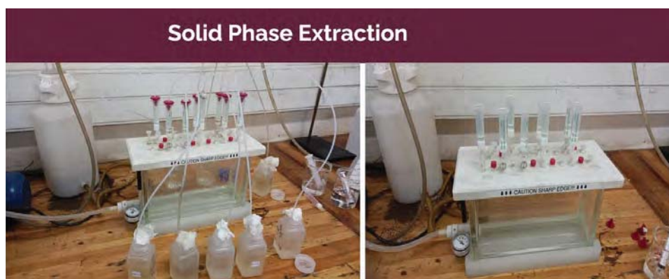
Figure 4-3: Solid Phase Extraction of PFAS from water samples under vacuum.
