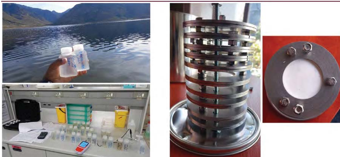
Figure 3-5: Grab sampling and passive sampler.
