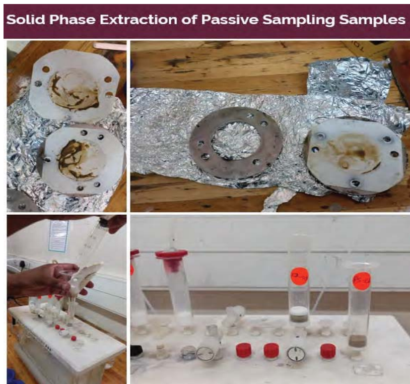
Figure 4-6: Solid Phase Extraction (SPE) of samples from passive sampling.
