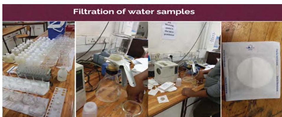
Figure 4-2: Filtration process of water samples.
