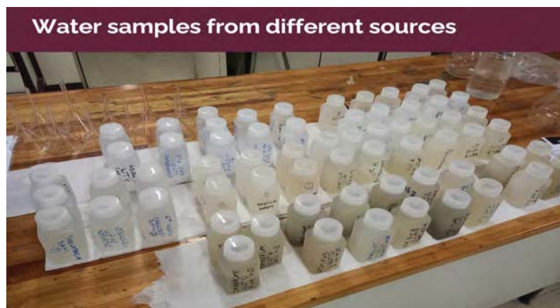
Figure 4-1: Spiked Water samples before SPE process.
