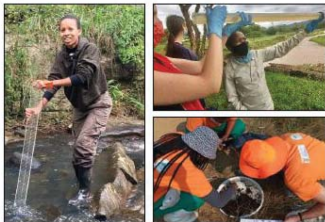
Left: Application of the Velocity Plank to measure stream velocity. Top right: Demonstration of Clarity Tube to school children. Bottom right: Rovers identifying macro invertebrate from the miniSASS sample.
