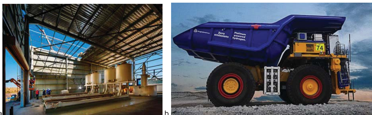
Figure 3.53 Electrolyser plant and hydrogen truck at Mogalakwena (Anglo American Platinum, 2022)
