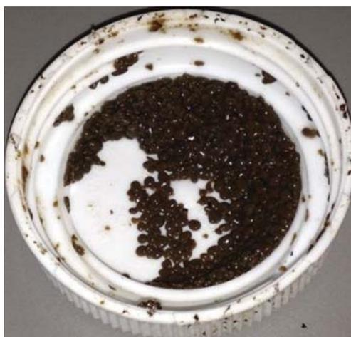
Figure 3-2 Granular sludge used as inoculum
