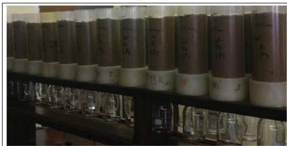
Figure 9.2: The ensemble that was utilised for the percolation and collection of the synthetic acid mine water that was passed through sand columns containing limestone
