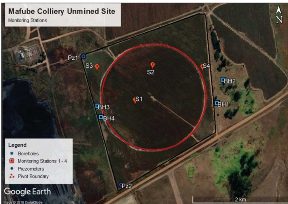
Figure 2.1: Monitoring stations on Mafube unmined land. The letter S denotes soil monitoring stations, BH refers to borehole monitoring sites, and Pz to piezometers.
