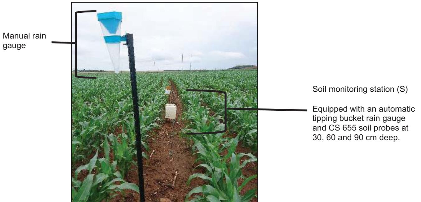
Figure 2.2: Typical field monitoring station setup at the dryland and pivot sites. An automatic and manual rain gauge, as well as the waterproof enclosure to house a data logger and battery for automated soil water and salinity measurements of the profile can be seen.
