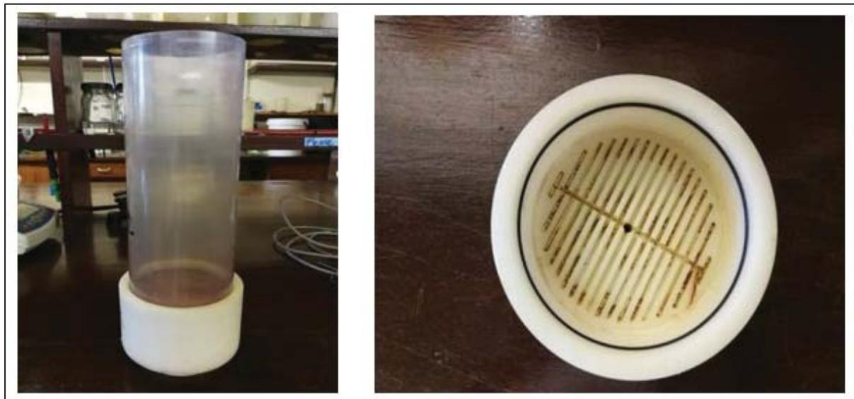
Figure 9.1: The column ensemble, which consists of a polyethylene tube and its base, with a gridded sieve to allow leachate to exit the column and prevent the loss of soil
