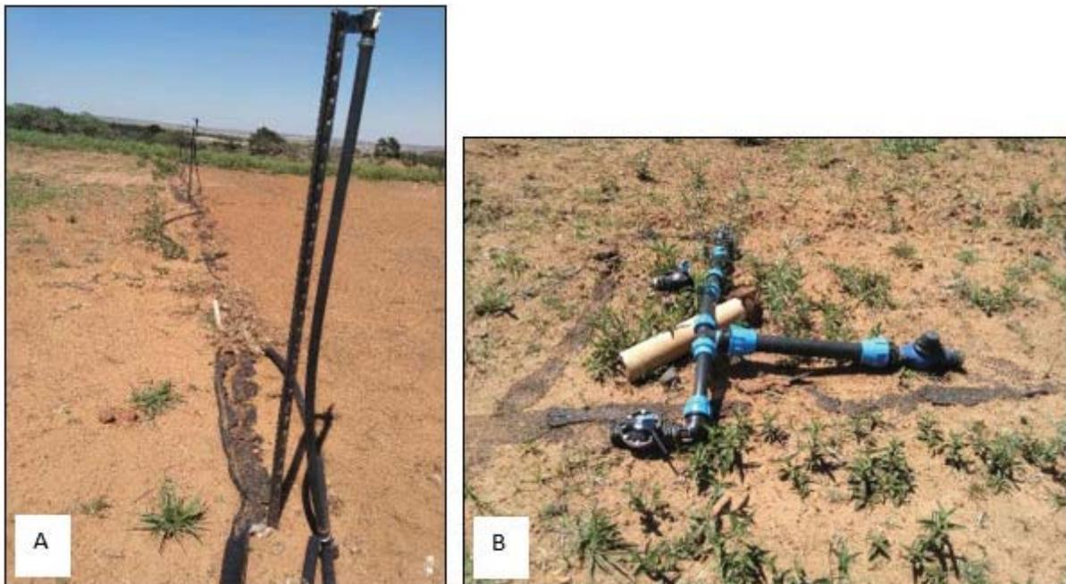
Figure 5.10: Fire melted A) pipes and B) connectors
