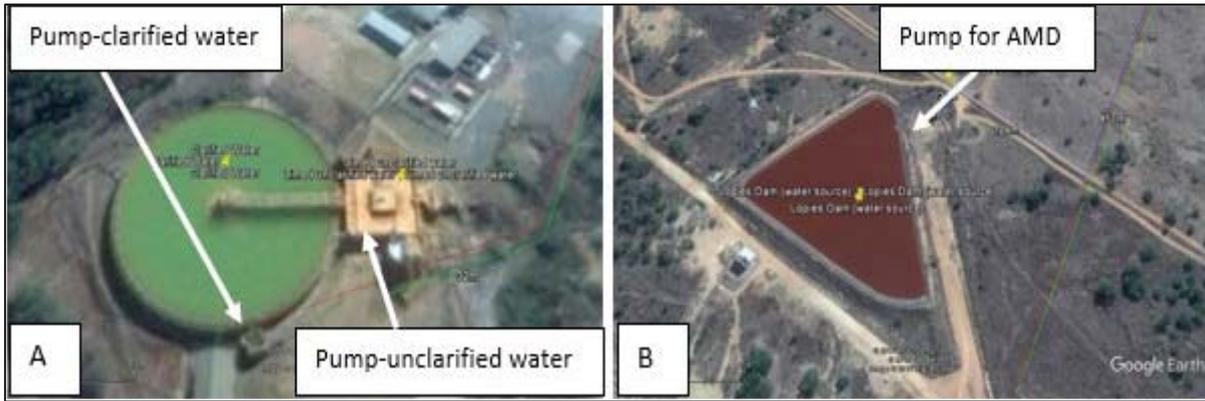
Figure 5.8: Sites for the installation of pump units: A: Sources of neutralised mine water (clarified and unclarified); B: Acid mine drainage (Lopies Dam)
