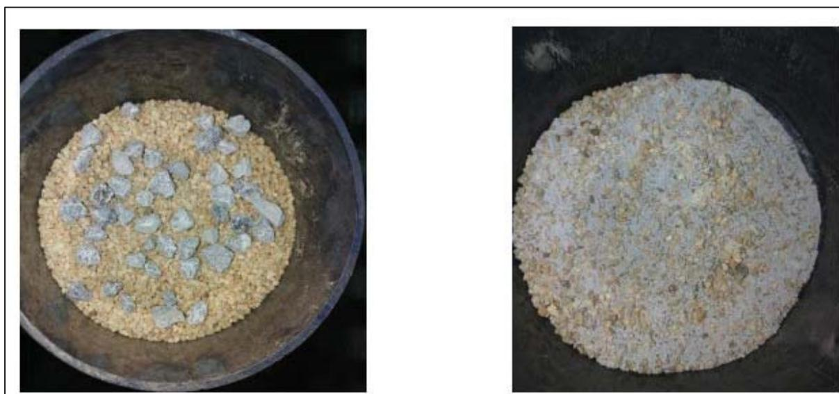
Figure 9.3: Surface application of 12.6 g limestone with a particle size of larger than 4 mm, but less than 10 mm (left) and less than 0.1 mm (right)
