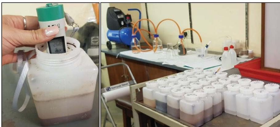
Figure 10.2: Samples after measurements were taken, before daily aeration; (ii) daily measurements using an ORP probe
