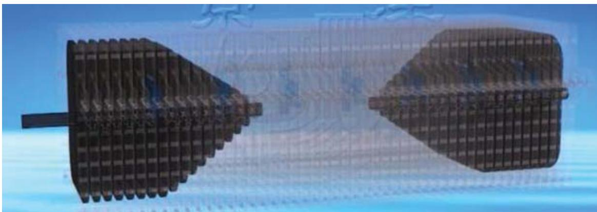
**Figure 37: Filter press receiving feed from both fixed and movable head sides simultaneously**
