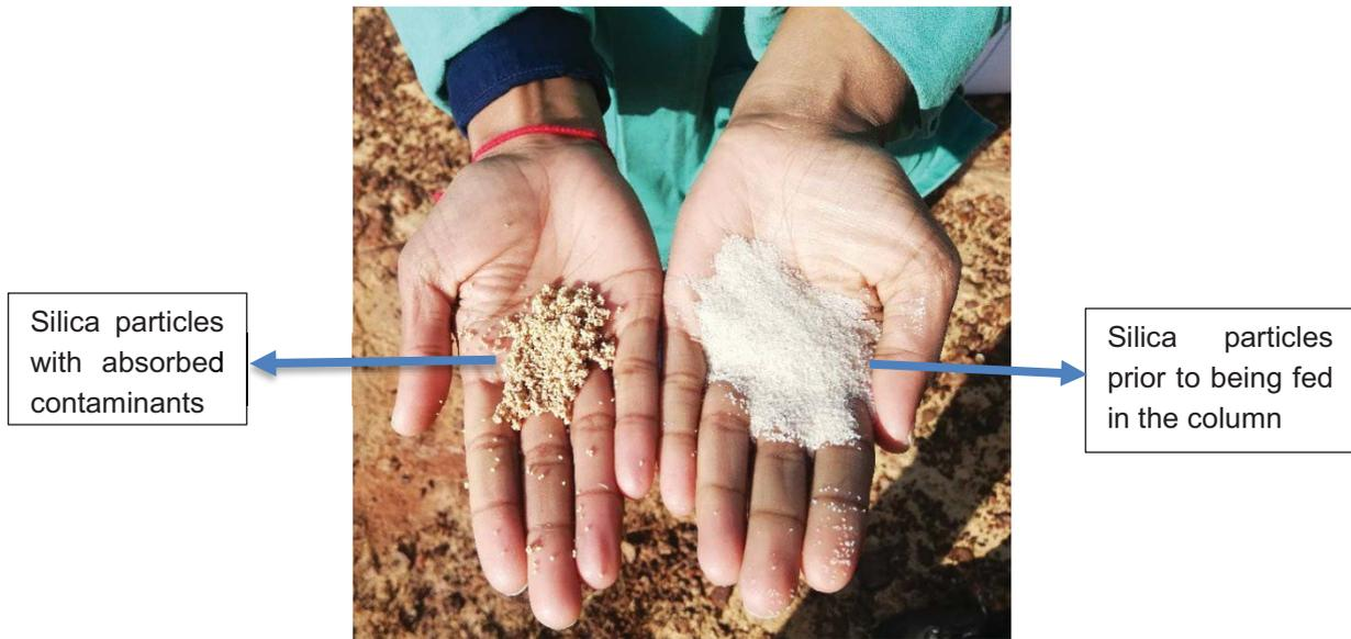
**Figure 51: Silica Particles after and before surface absorption**
