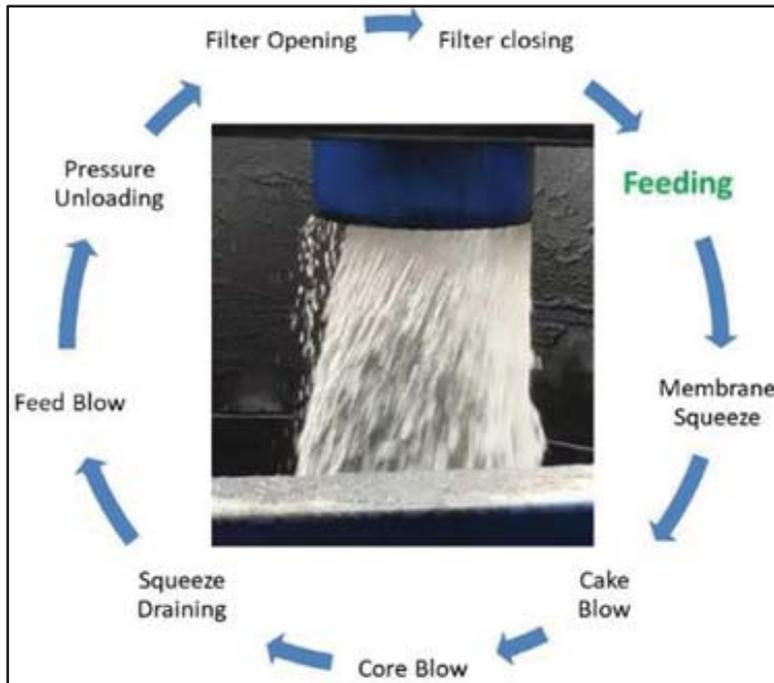
**Figure 39: Steps included in the plate and frame filter press cycle**
