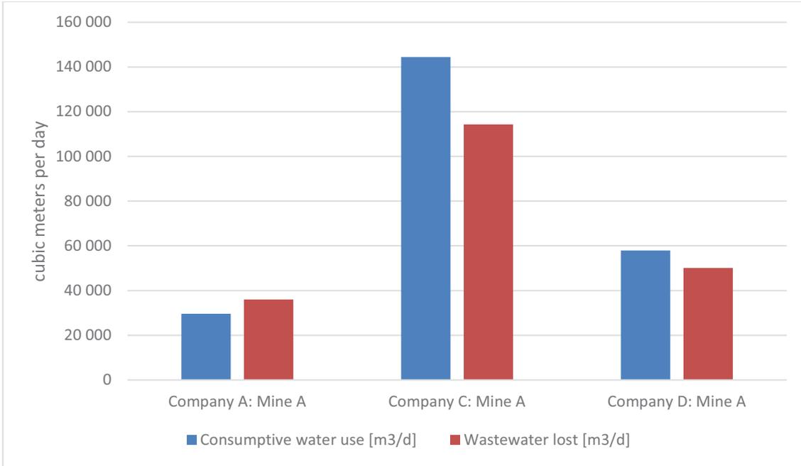
Figure 17: Consumptive water use and wastewater lost for some Platinum mines
