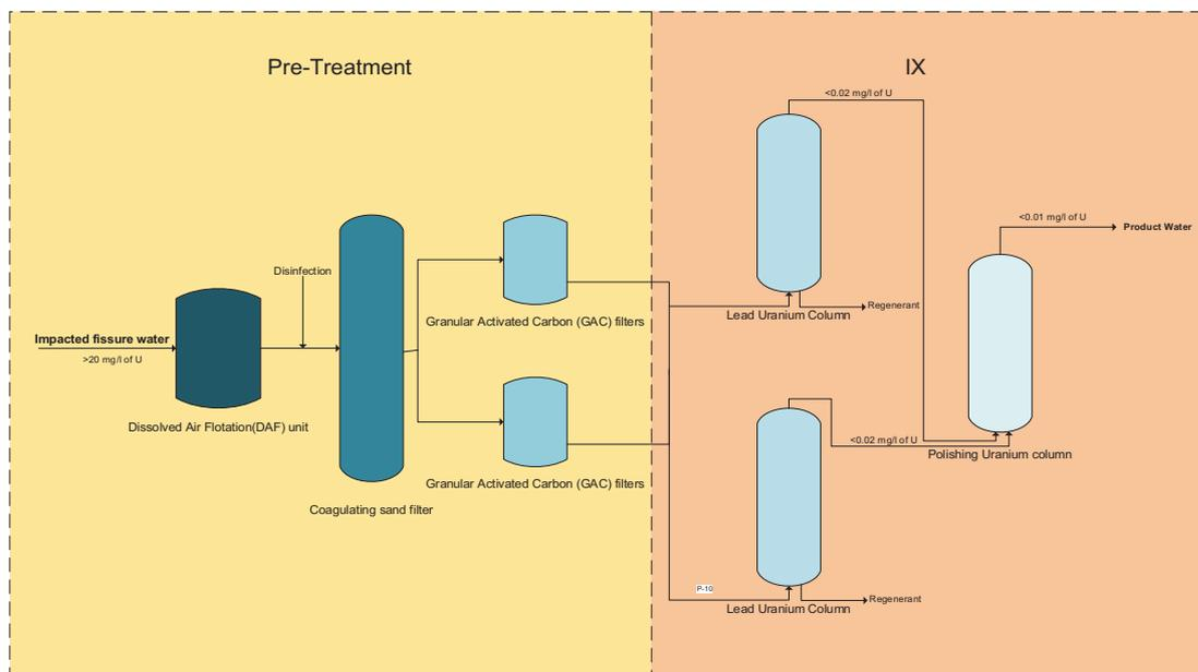
Figure 55: IX process flow diagram ( Botha. M., 2009)
