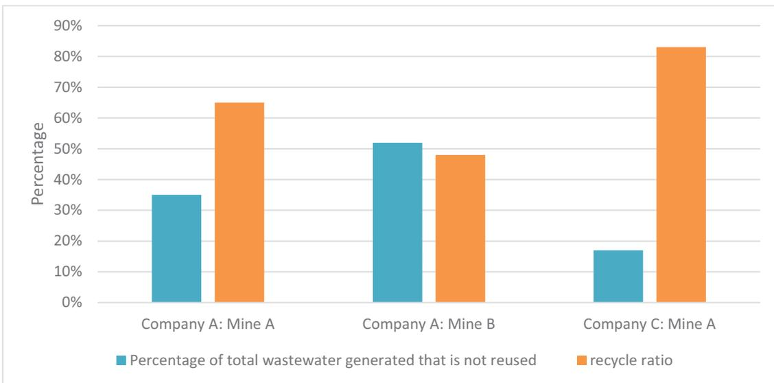
**Figure 16: Percentage wastewater not re-used and recycle ratio for some Gold mines**
