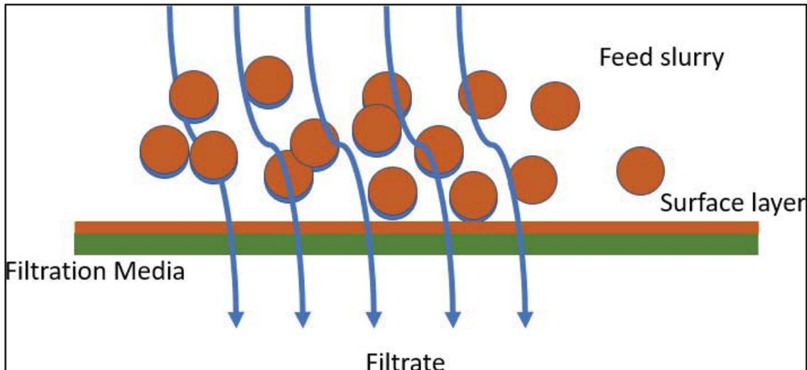
**Figure 40: Filtration Principle – Selectively permeable membrane (ENPROTEC)**
