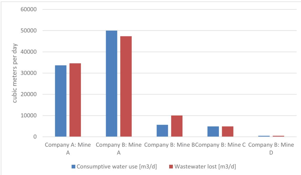
**Figure 20: Consumptive water use and wastewater lost for some Diamond mines**
