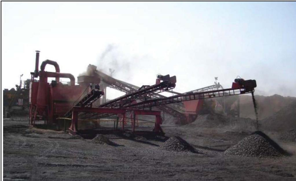
**Figure 32: Xantium FGX unit at Palesa Colliery (de Korte, 2010)**
