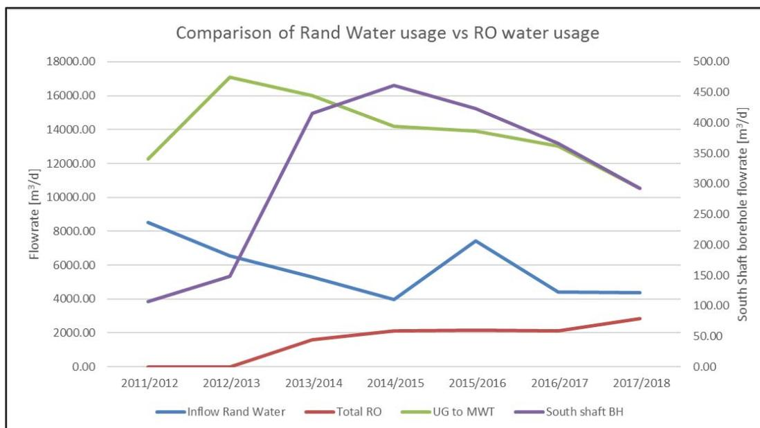
**Figure 44: Comparison of Rand water vs RO water usage over the years**
