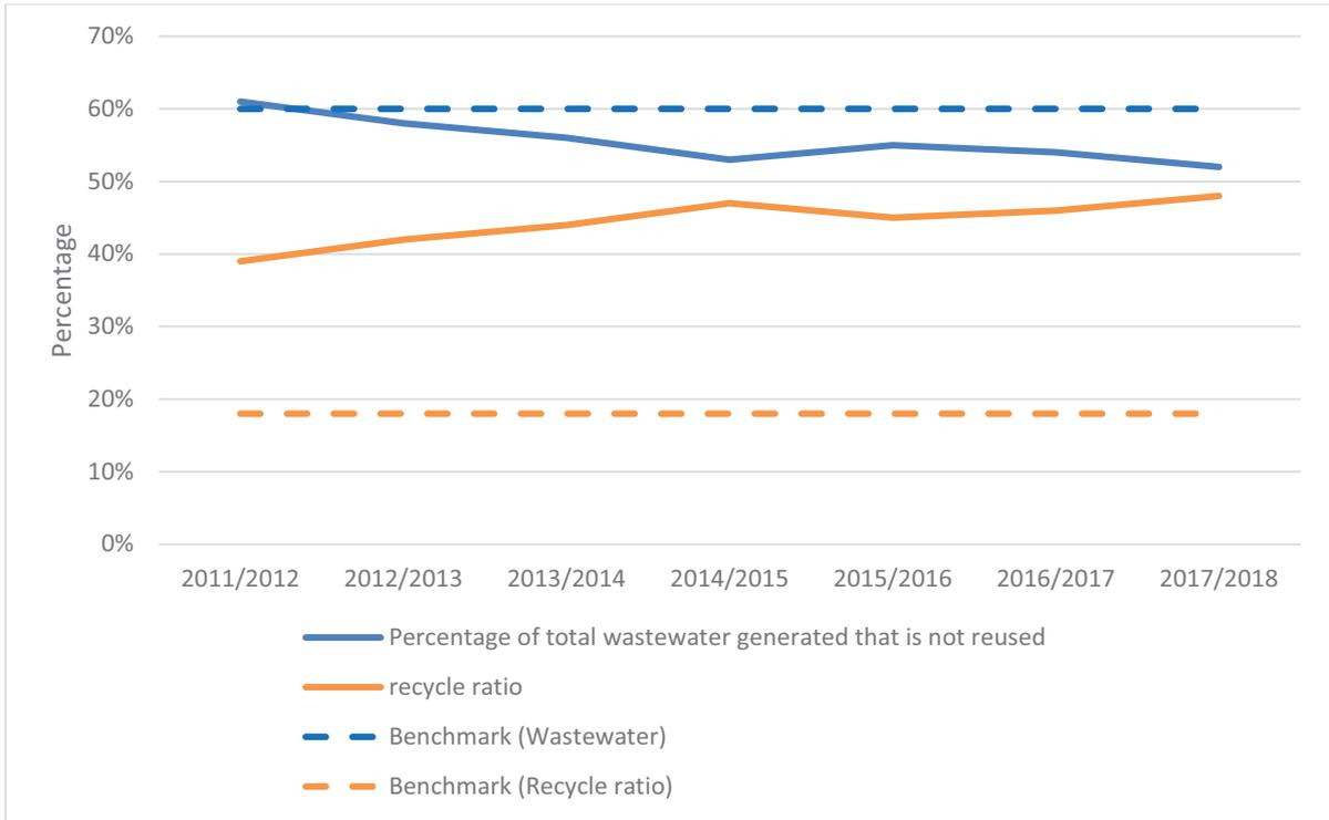
**Figure 47: Percentage of wastewater lost that is not re-used and recycle ratio**
