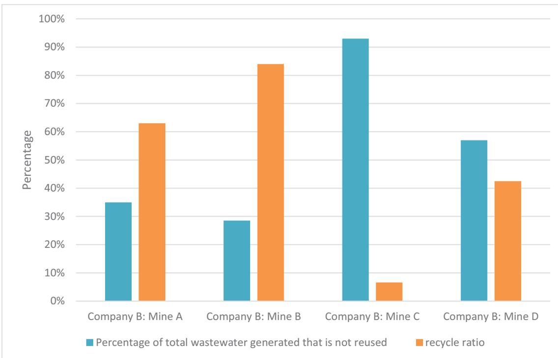
**Figure 22: Percentage wastewater not re-used and recycle ratio for some Diamond mines**
