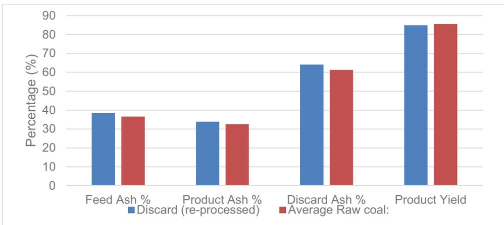
**Figure 33: Results obtained from the Xantium FGX**
