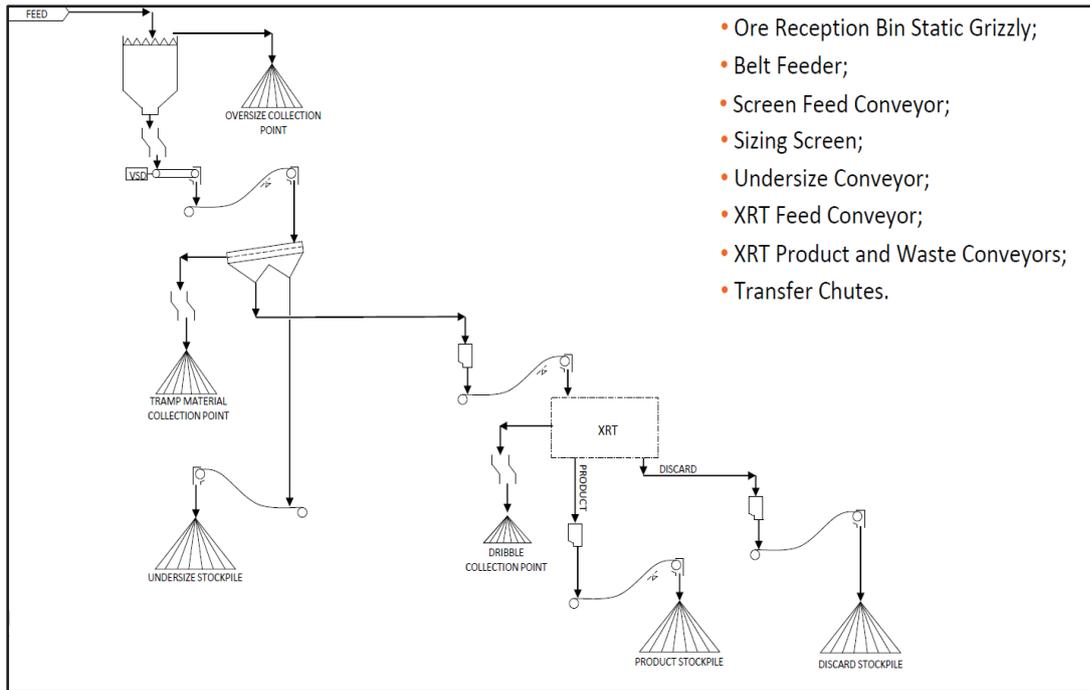
**Figure 41: Process flow diagram**
