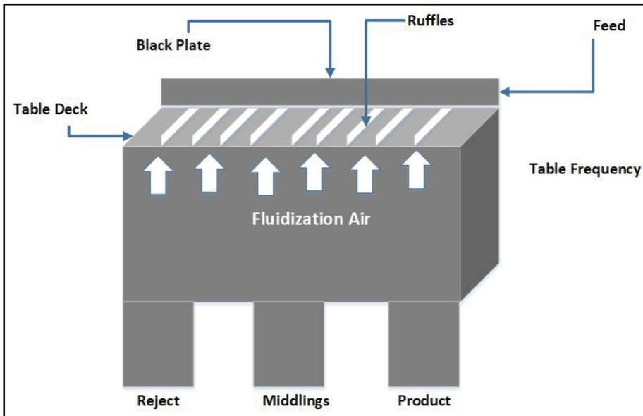
**Figure 26: Simplified process diagram of the FGX plant**
