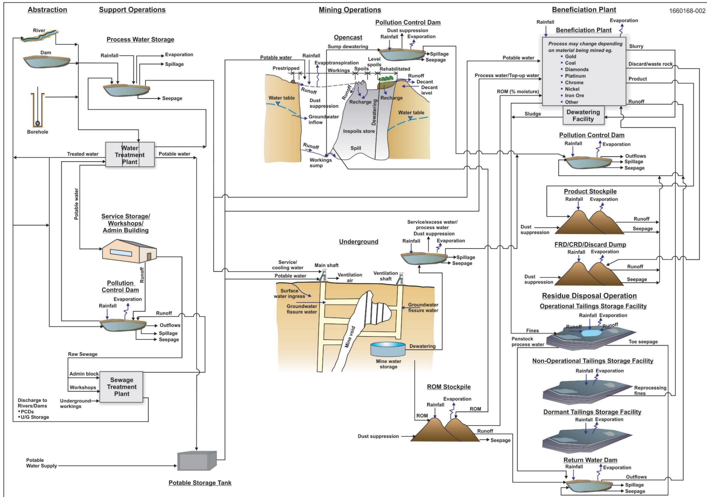
Figure 4: Generic mine water reticulation diagram
