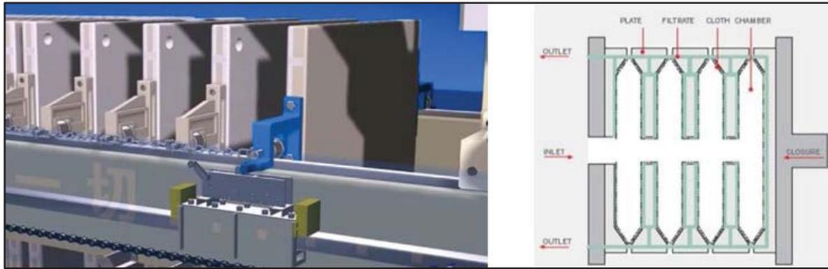
**Figure 35: Plate and frame filter press showing, a) concave filter pates and, b) cavity that forms between successive plates (<http://www.lenntech.com>)**
