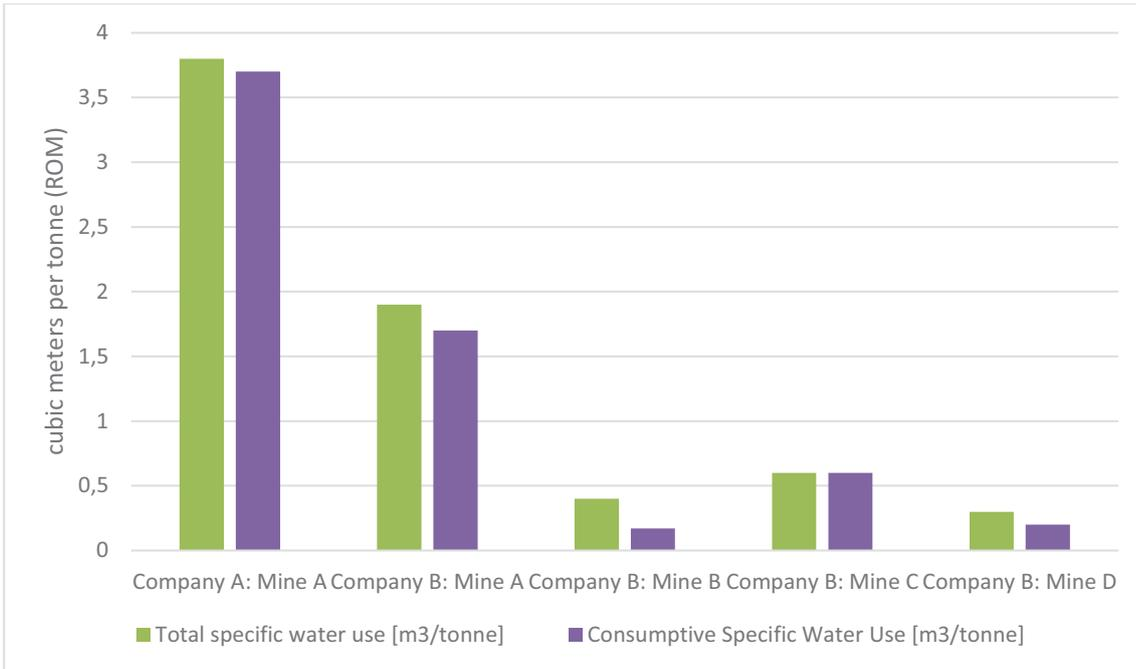
**Figure 21: Total specific and consumptive specific water use for some Diamond mines**
