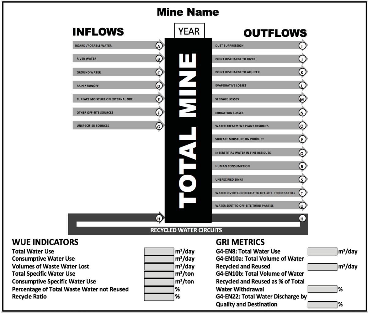
Figure 7: Flow diagram to illustrating the calculation of WUE indicators (DWS, 2016b)
