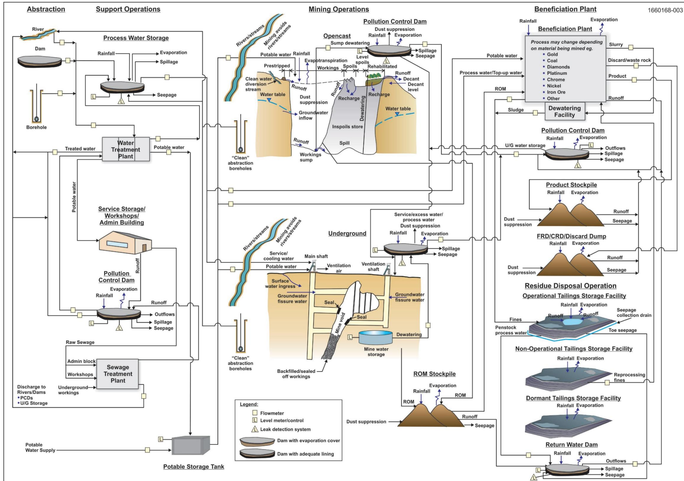
Figure 5: Some WC/WDM interventions on a typical mine site-wide reticulation diagram
