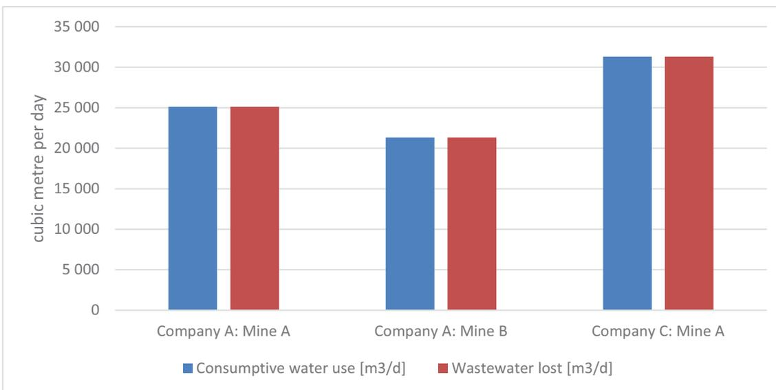
**Figure 14: Consumptive water use and wastewater lost for some Gold mines**
