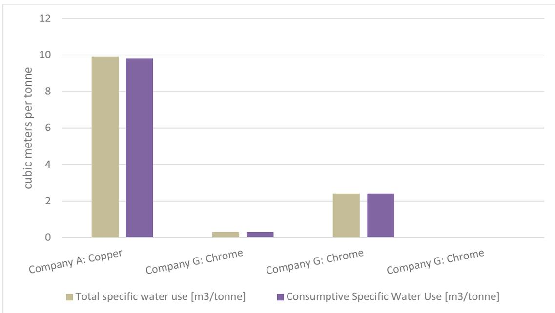
**Figure 24: Total specific and consumptive specific water use for some Copper and Chrome mines**
