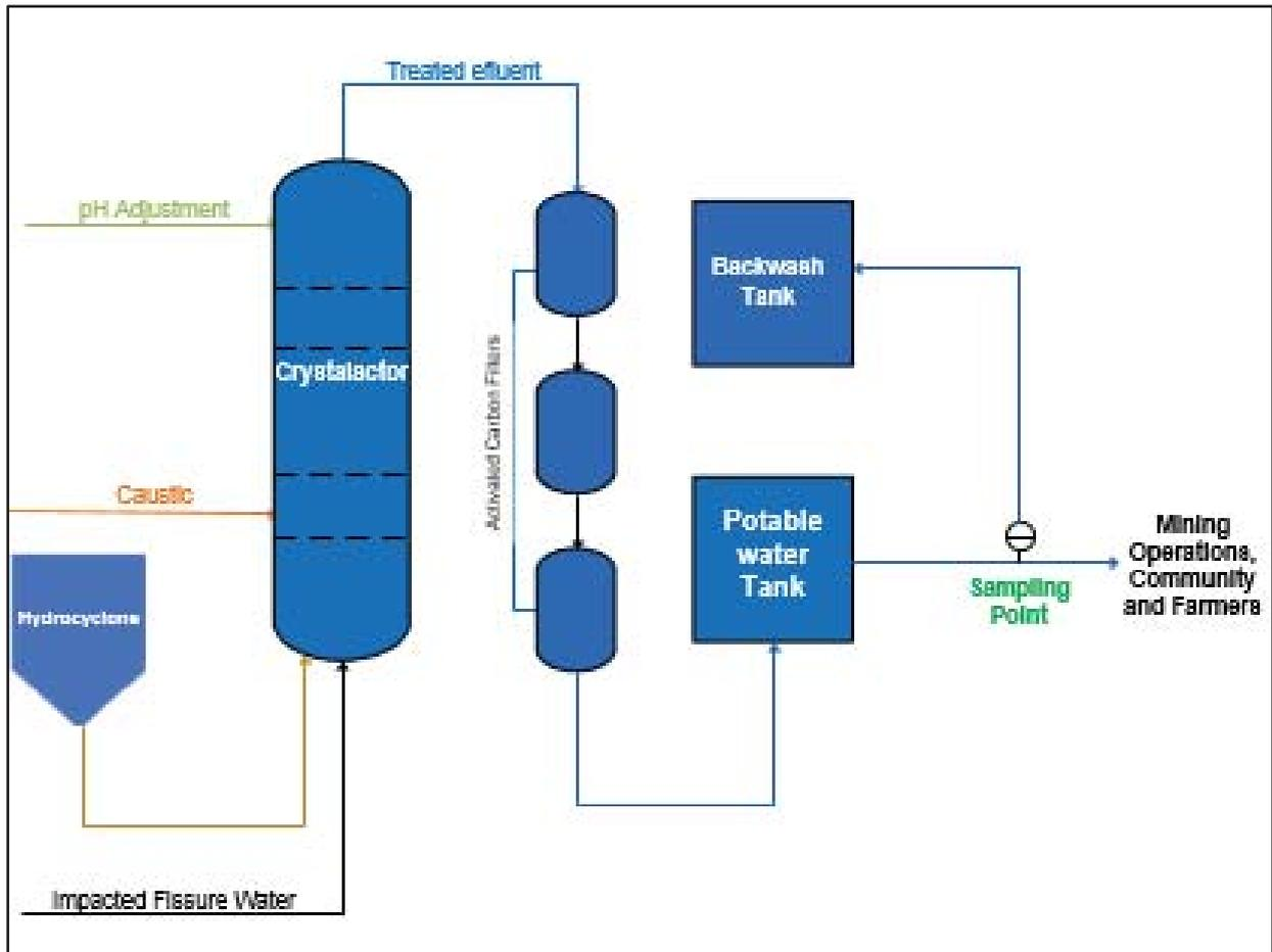
Figure 50: Simplified process diagram of Crystalactor plant at Mine W plant
