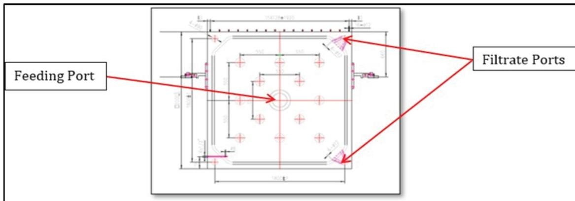
**Figure 36: Filter press plate showing feeding and filtrate ports**
