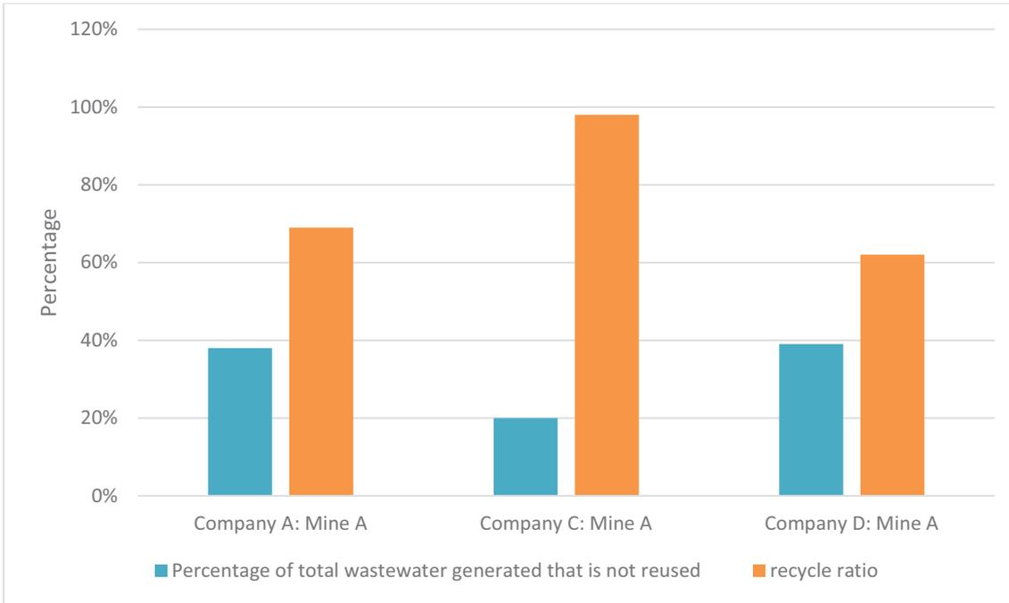
**Figure 19: Percentage wastewater not re-used and recycle ratio for some Platinum mines**
