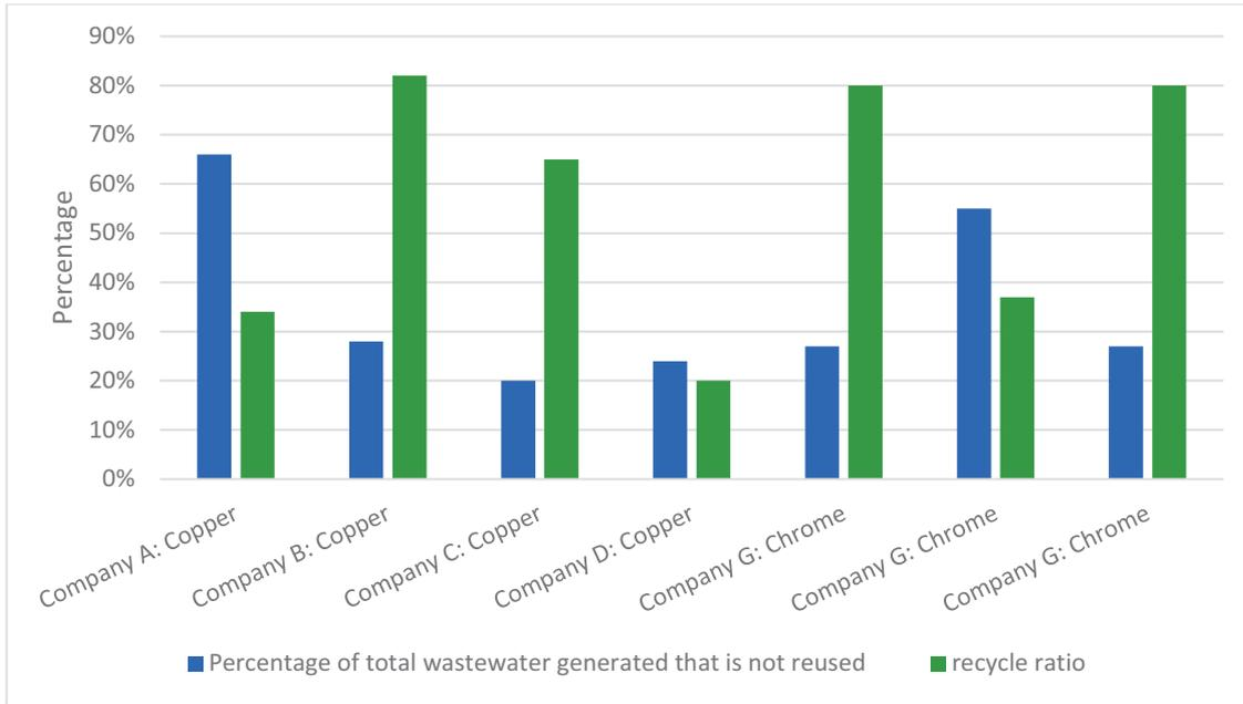
**Figure 25: Percentage wastewater not re-used and recycle ratio for some Copper and Chrome mines**
