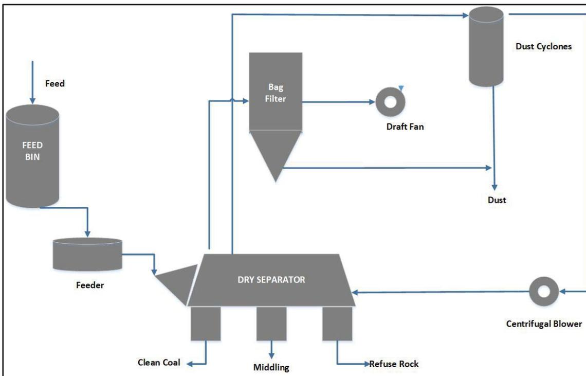
**Figure 27: Typical FGX plant layout**
