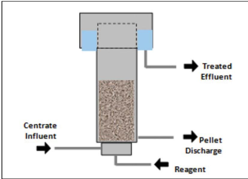
**Figure 49: Crystalactor Technology operating principle**
