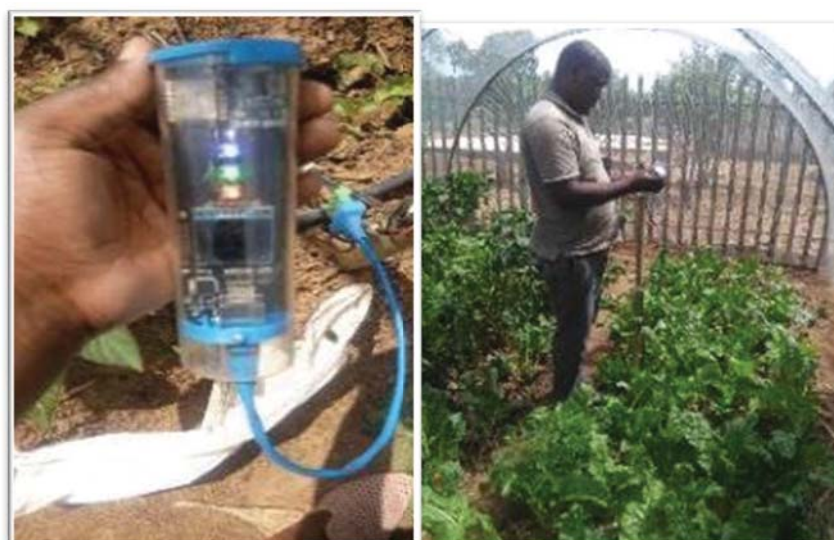
Figure 19: Right; An example of a Chameleon sensor in this case indicating blue, green and red for the three different soil depths (20, 40 and 60 cm respectively) Far right; Sylvester Selala in Christina's tunnel checking the sensor.
