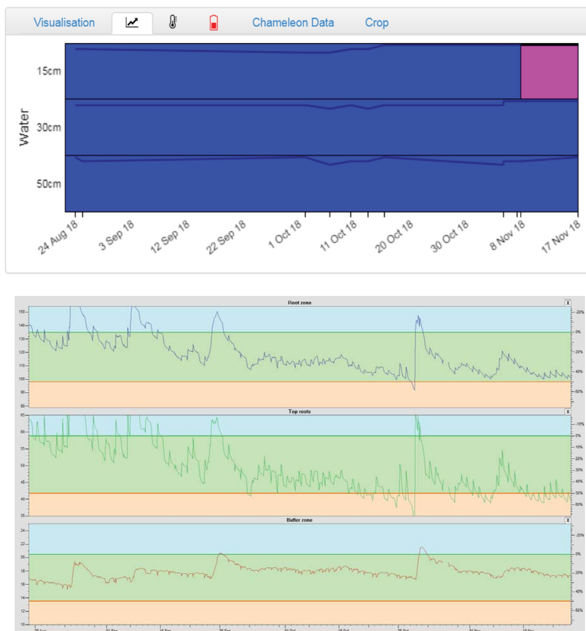
Figure 7.13: Chameleon sensor data for three soil layers (15, 25 and 40 cm) (top graph) and DFM soil water contents (bottom composite graph) for the total root zone (top pattern), top roots (middle pattern) and buffer zone (bottom pattern) of field KD2 West.
