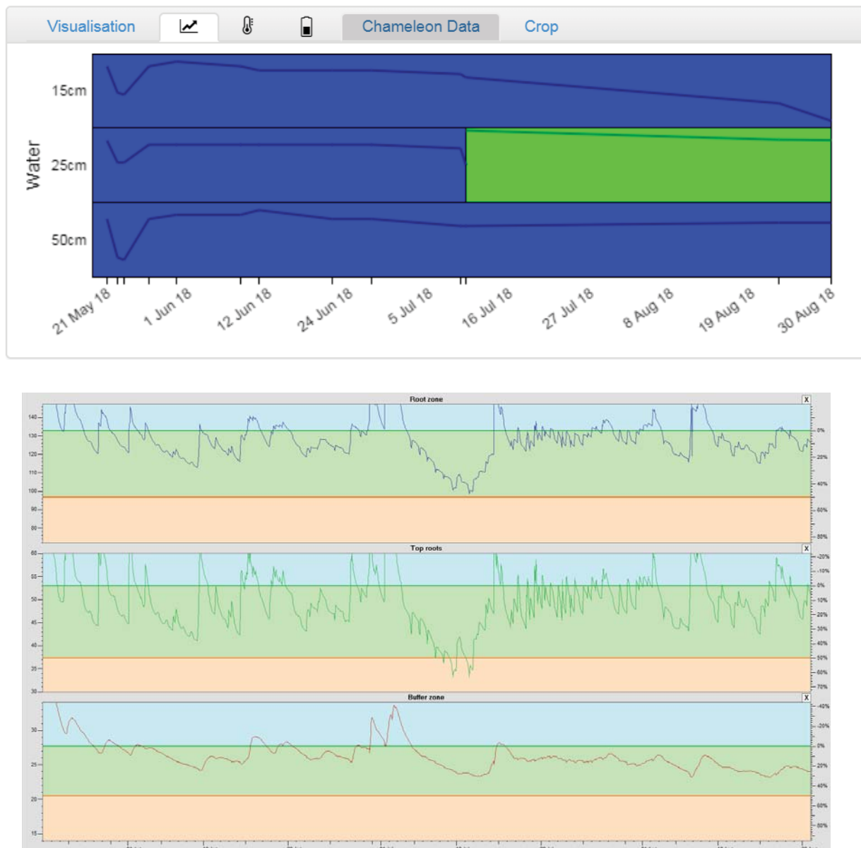
Figure 7.11: Chameleon sensor data for three soil layers (15, 25 and 40 cm) (top graph) and DFM soil water contents (bottom composite graph) for the total root zone (top pattern), top roots (middle pattern) and buffer zone (bottom pattern) of field RF12 Bottom.
