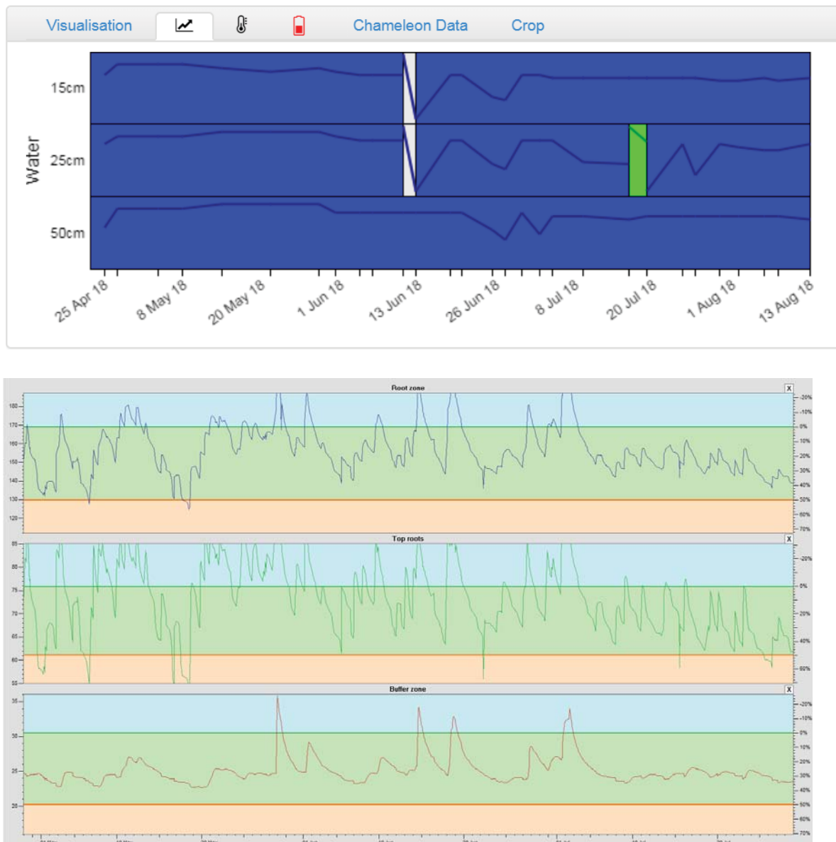
Figure 7.9: Chameleon sensor data for three soil layers (15, 25 and 40 cm) (top graph) and DFM soil water contents (bottom composite graph) for the total root zone (top pattern), top roots (middle pattern) and buffer zone (bottom pattern) of field 10B East.
