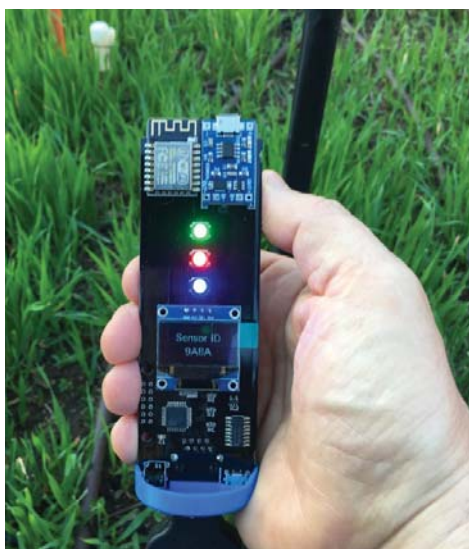
Figure 1.2: Chameleon field reader indicating different coloured lights
