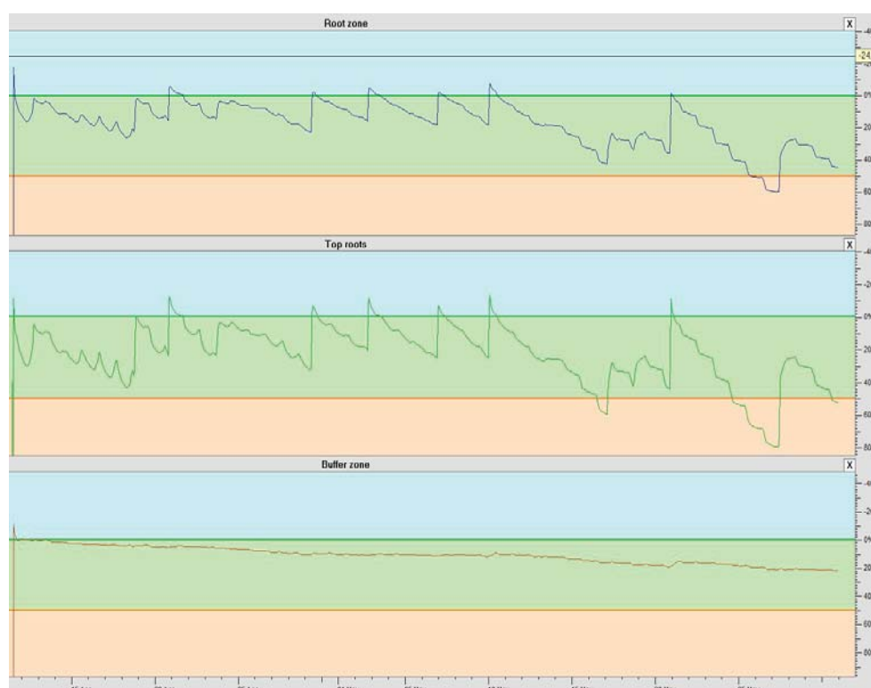
Figure 7.3: DFM soil water patterns for potatoes (field M8 – loam), Dendron, 2017. Top section of graph shows water content of the total root zone (0-40 cm), while middle section shows the top roots (0-20 cm) and bottom section shows the buffer zone (40-60 cm).
