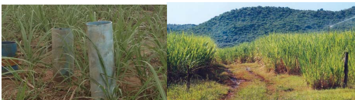
Figure 9.3: Chameleon sensors installed in young (left) and matured (right) sugarcane
