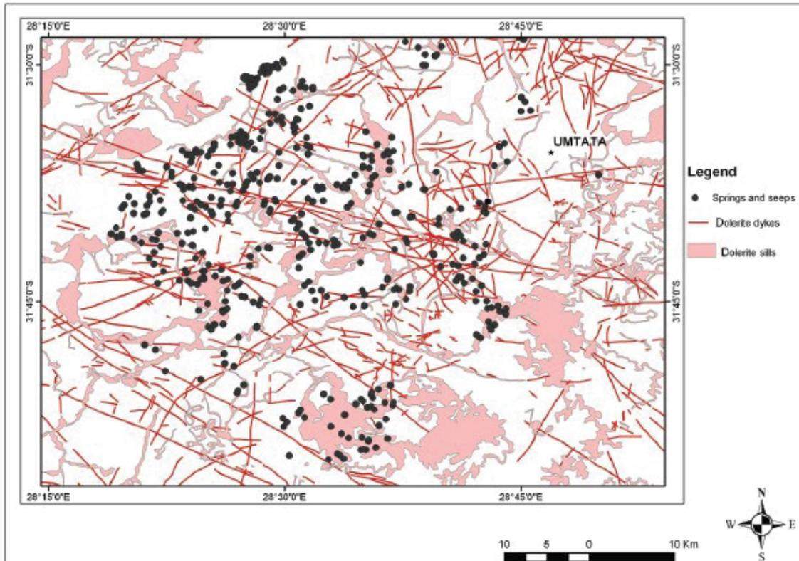
**Figure A10:** Distribution of springs and dolerite dykes and sills, west of Mthatha (from Dondo et al., 2010).
