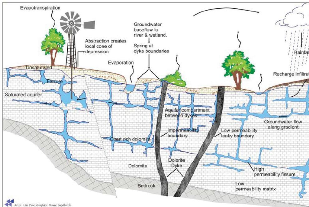
**Figure A8:** Schematic cross-section of the dolomitic aquifer of North-West Province, South Africa (from Colvin et al., 2007).
