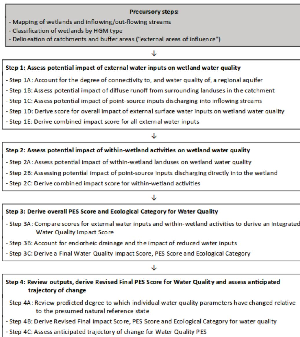
Figure 9.3. An outline of the steps involved in the application of the Water Quality module
