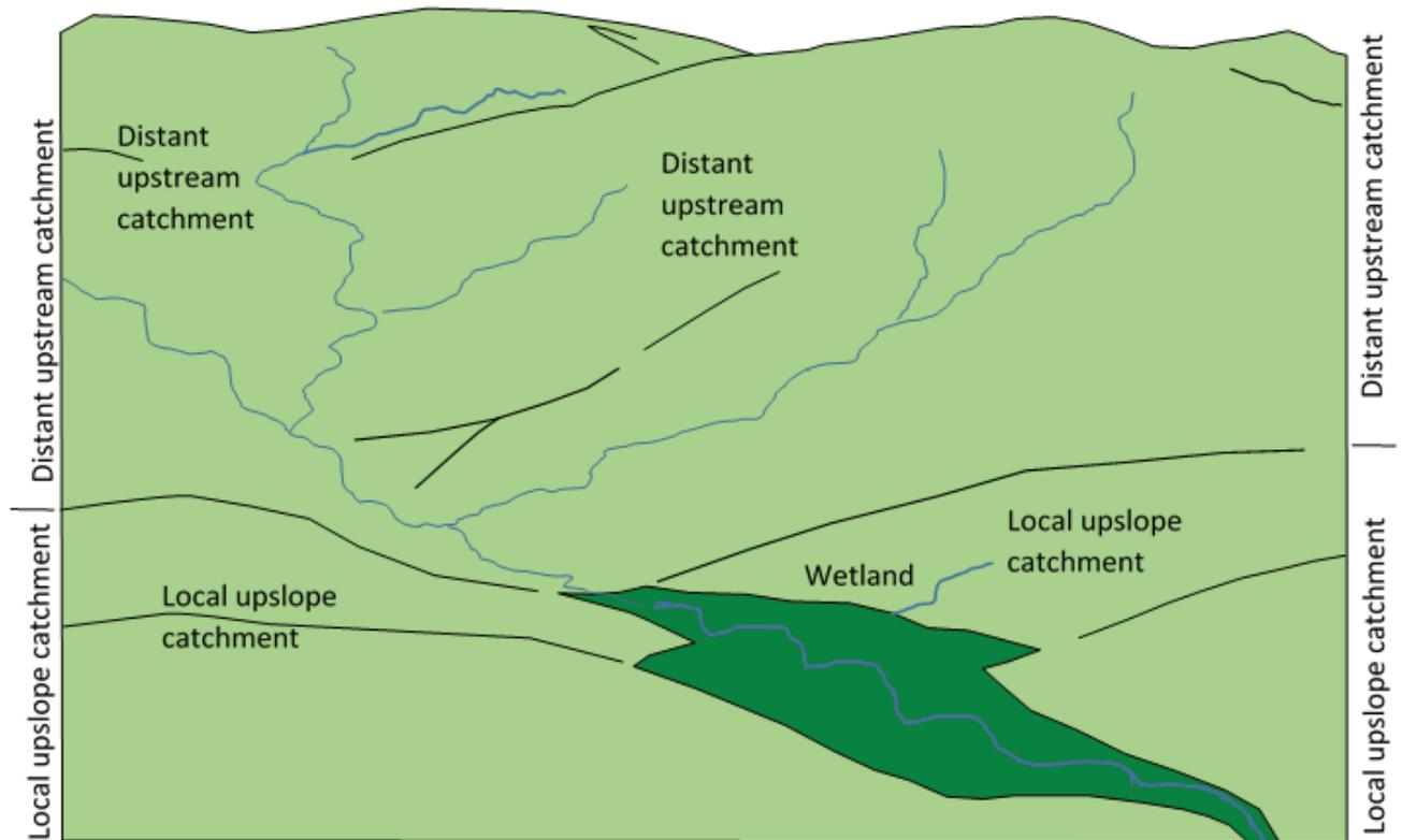
**Figure A2:** A wetland and its local upslope catchment and distant upstream catchment
