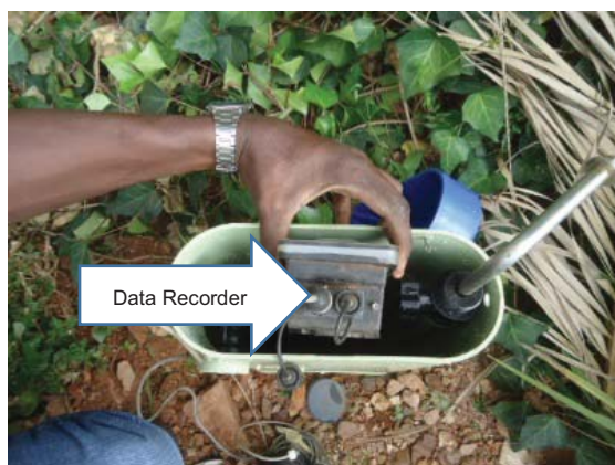
Inserting data recorder into meter box
